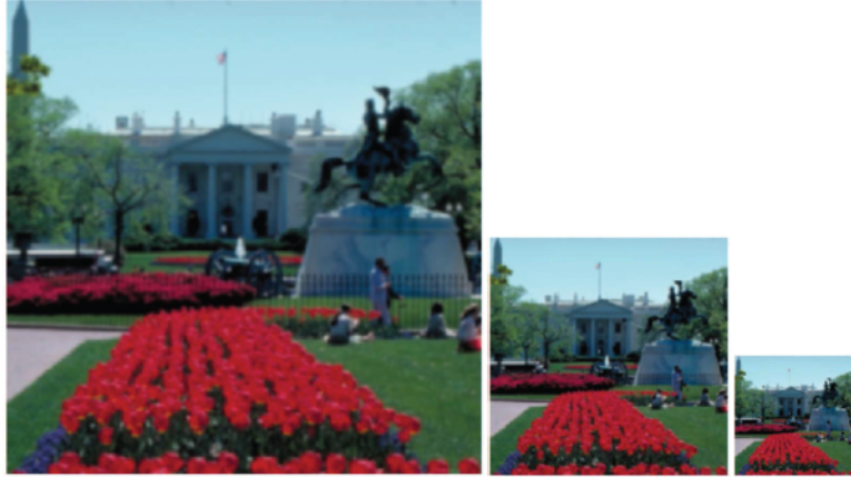
Figure 3.3: Impact of image resolution on sharpness. From left to right: Original image, images down-sampled by 2\times and 4\times respectively.
