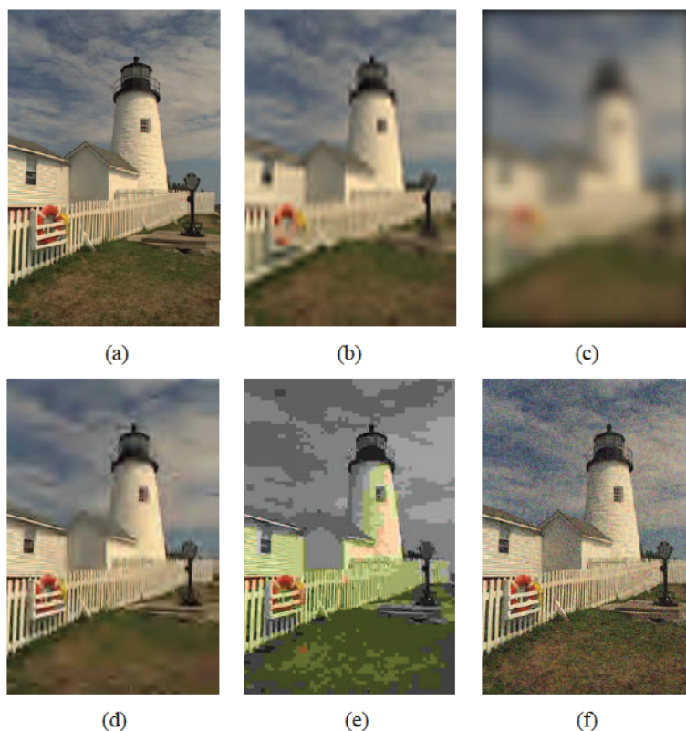
Figure 1.5: A pristine image and five distorted counterparts. (a) Pristine image. (b) Rayleigh fast fading. (c) Gaussian blur. (d) JPEG2000 compression. (e) JPEG compression. (f) White noise. Images are from the LIVE database [18].
