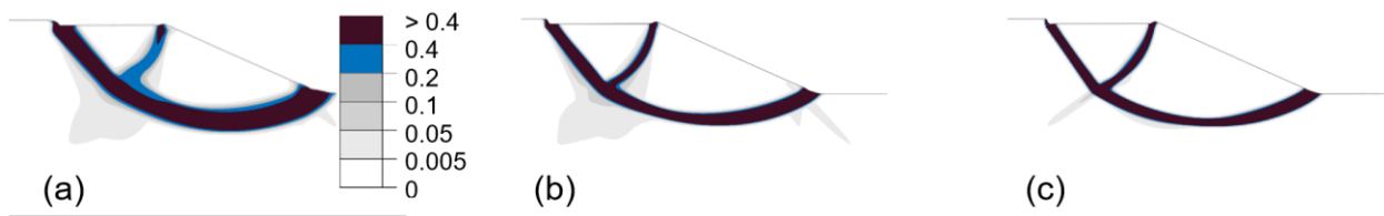
Figure 4.10 Local deviatoric plastic strain contours of over-nonlocal models with softening scaling: (a) l = 0.25 m; (b) l = 0.125 m; (c) l = 0.0625 m
