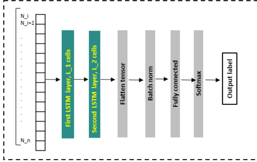
Figure 6.1: Overview of the proposed LSTM sequential data based CTC detection model.
