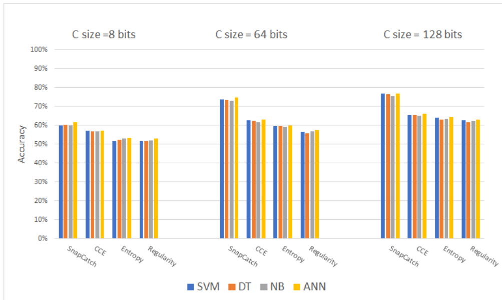
Figure 4.8: The impact of the covert message size on the detection accuracy of UCCTC in WAN network.
