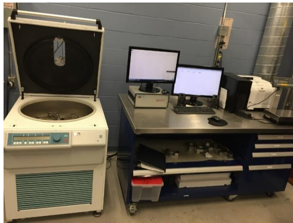
Figure 8 Ultra-centrifuge machine in Hibernia Enhanced Oil Recovery (EOR) Laboratory
