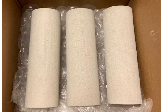
Figure 23 Cores that are used for centrifuge experiments in Homogeneous Case 1
