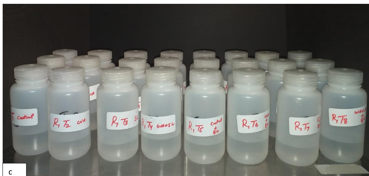
Figure 3.1 (a-c): Leaching column experiment setup with collected leachate.
