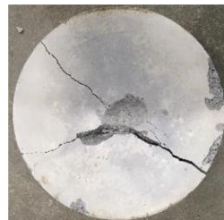
Typical crack pattern for BPVA and BSF cylindrical composites
