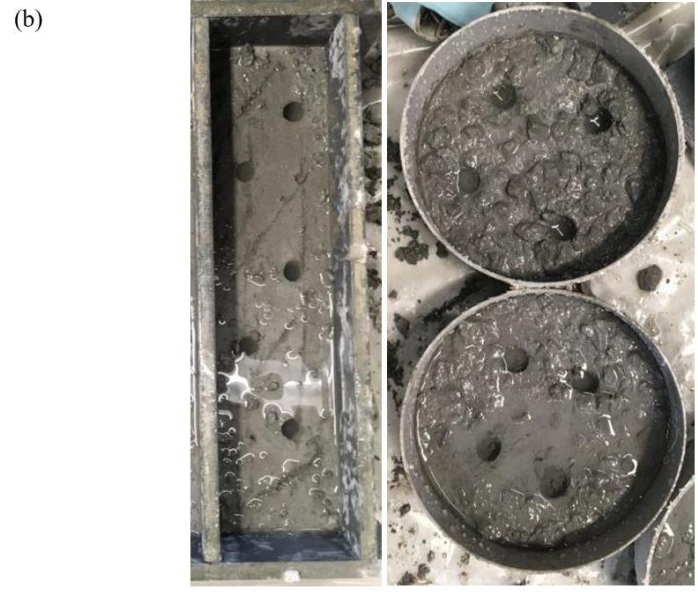
Figure 4-4 (a) Configurations of cast composites (b) preparation before casting the top layer
