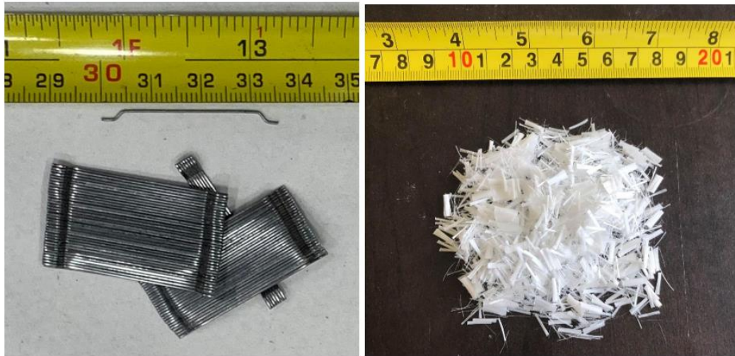
Figure 3-2 Geometry and configuration of fibers used
