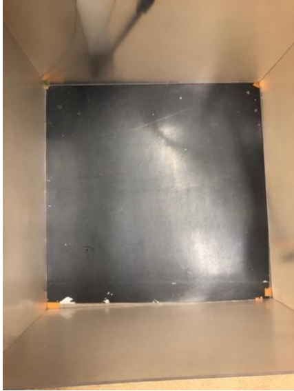
Figure 3. Open Field Maze apparatus. Dimensions are 60 x 60 x 50 cm.
