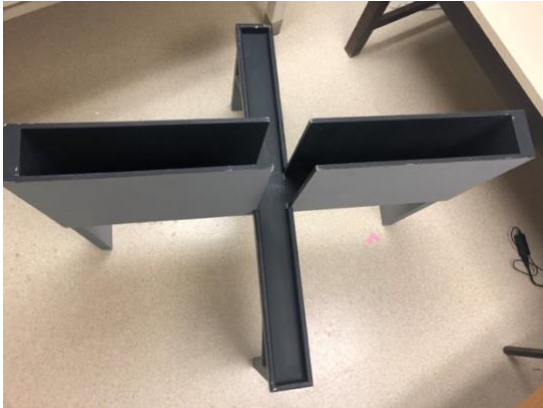
Figure 2. Elevated Plus Maze apparatus. Arms are 50 x 10 cm, walls on closed arms are 38 cm high, center platform is 11 x 11 cm, and it is raised 52 cm off the ground.
