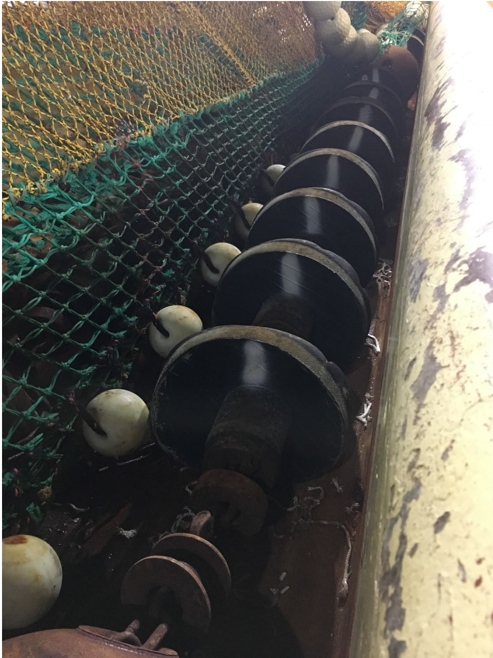
Figure 1.5. A typical roller footgear used in Eastern Canada offshore Northern shrimp ( Pandalus borealis ) fishery.
