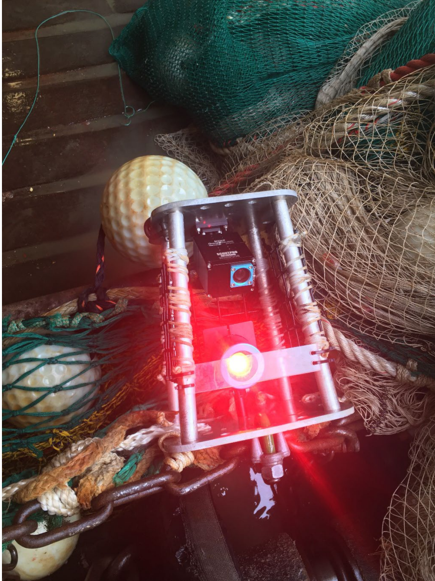
Figure 2.3. Video system attached to the fishingline above the port side quarter-wing footgear section.
