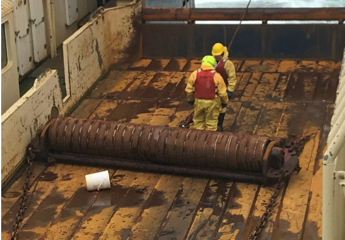
Figure 1.3. Roller clump in Eastern Canada offshore Northern shrimp ( Pandalus borealis ) fishery used for twin-trawling.
