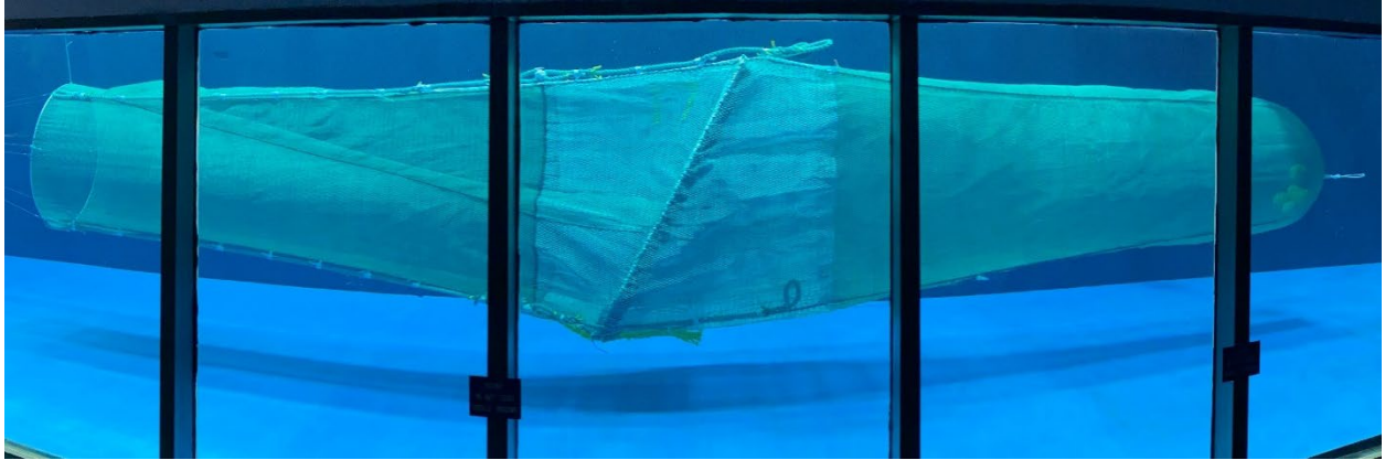
Figure 5.1. Traditional 22 mm bar spacing Nordmøre grid section during flume tank testing.
