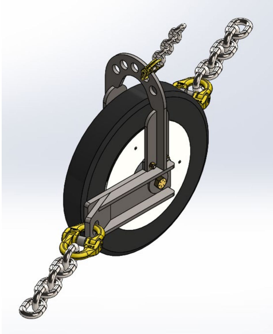
Figure 3.2. Schematic drawing of the full-scale prototype of an aligned-rolling wheel in SolidWorks.
