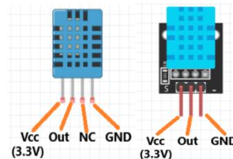
Fig. 4. The pin diagram of DHT11 temperature sensors.
