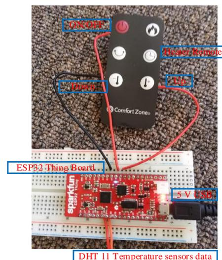
Fig. 14. Hardware connection of the proposed monitoring and control systems.
