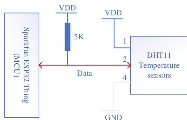
Fig. 5. The connection diagram of ESP32 and DHT11.
