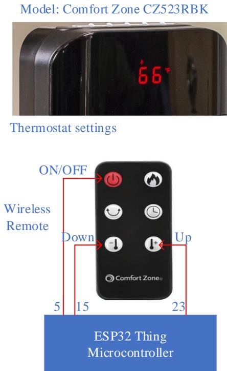
Fig. 8. The connection diagram of remote and ESP32 Thing for thermostat settings.
