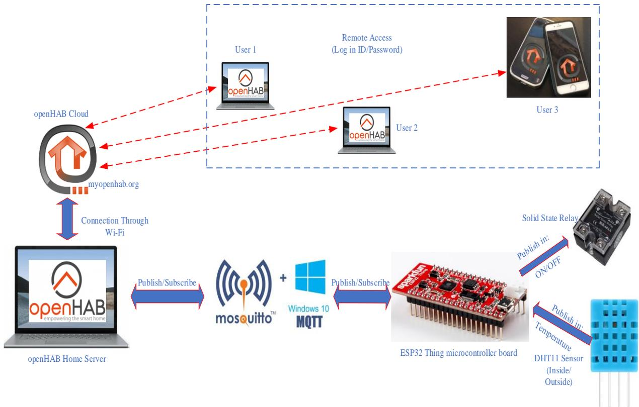
Fig. 13. The communication mechanism.
