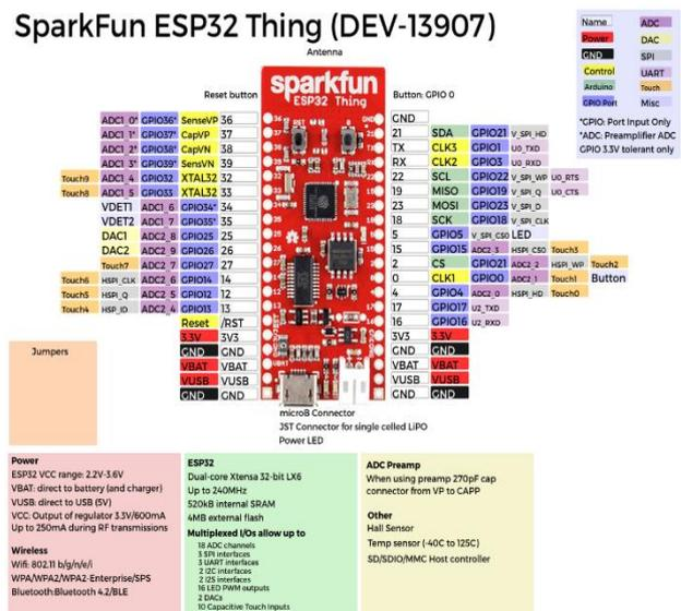
Fig. 7. The detailed architecture of the ESP32 Thing board.
