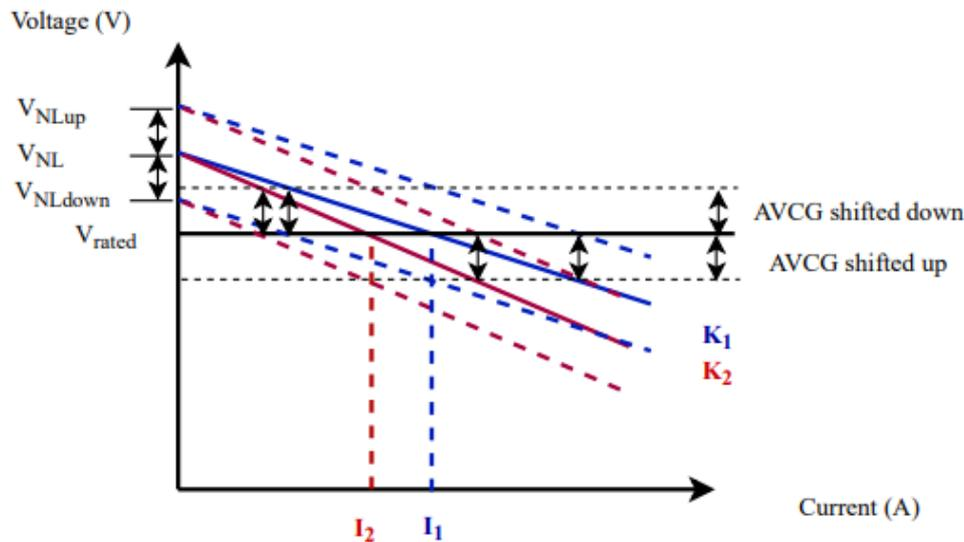
**Figure 8.** Load regulation characteristics of the droop method with AVCG implementation.
