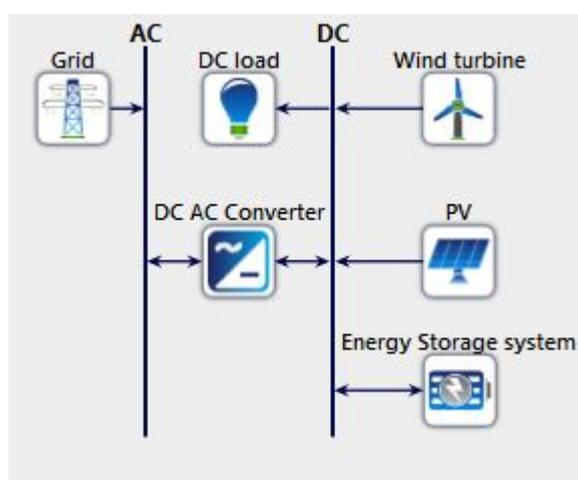
**Figure 1.** A typical configuration of a DC microgrid.
