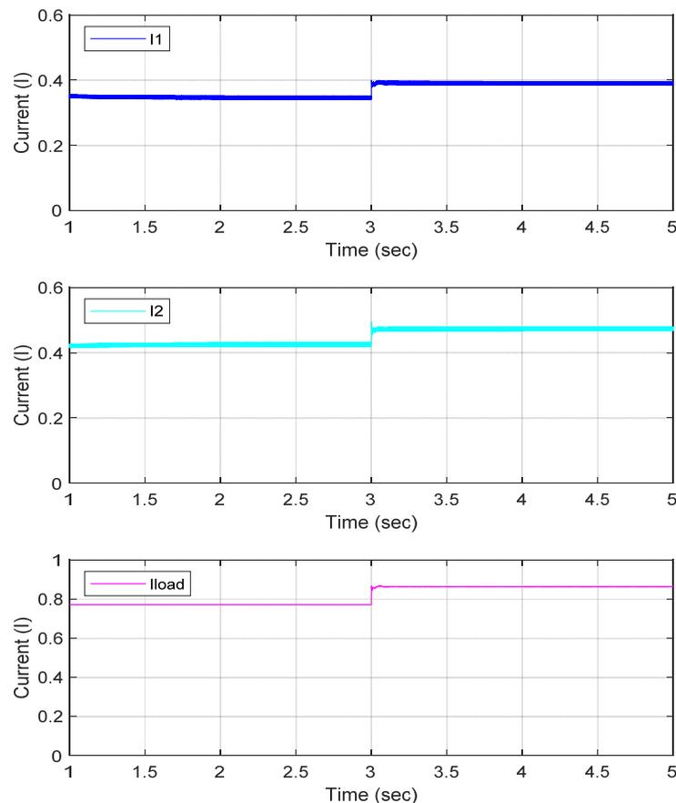
**Figure 10.** Simulation results of current sharing for a step increase in the load with the modified droop method.
