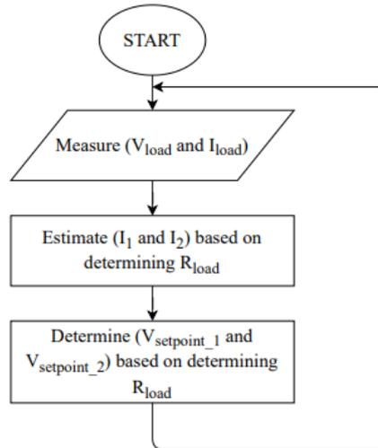
**Figure 5.** Flow chart of the modified droop control for determining the set point of each loop controller.
