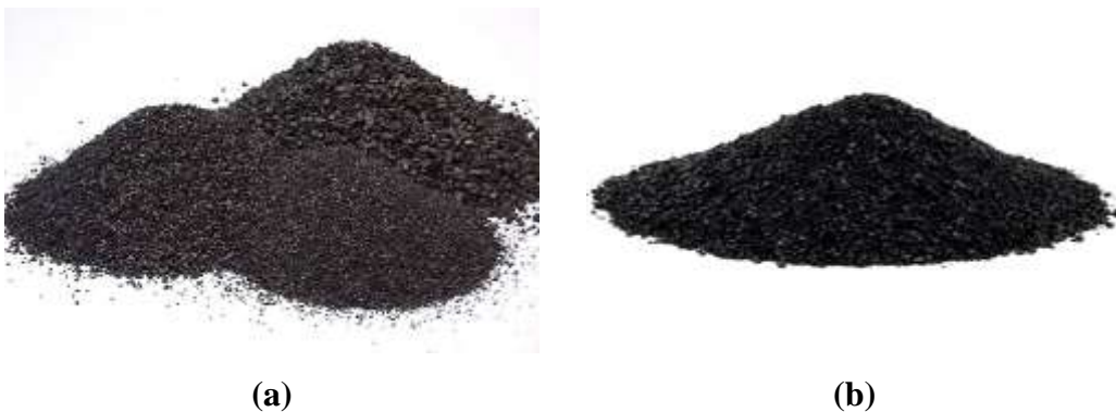
Figure 2.14: Representative illustrations of (a) steel slag (Adapted from “Steel slag briquetting machine,” n.d.); and (b) copper slag (Adapted from “Marco Abrasives-Copper Slag,” n.d.)
