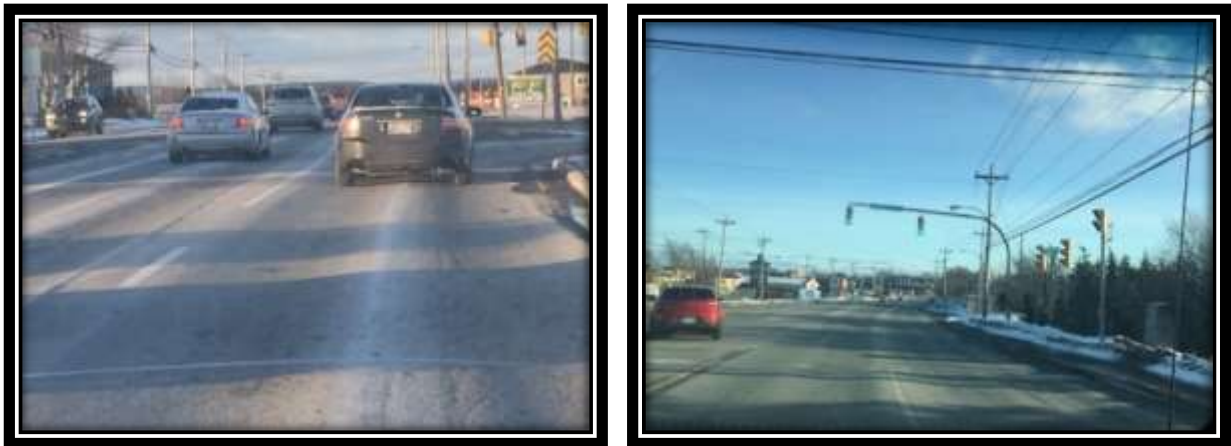
Figure 2.1: Asphalt design-related rutting (permanent deformation on wheel path) on Torbay and Stavanger (left) and Torbay and Gleneyre (right), St. John's
