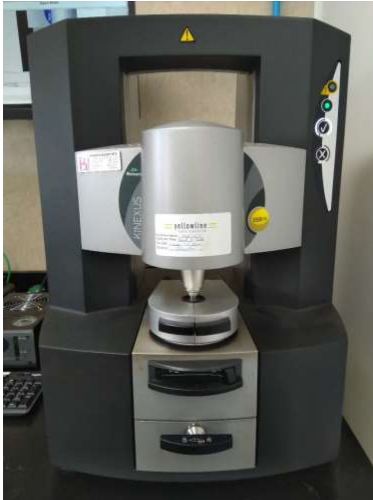
Figure A.6: A Malvern Panalytical Kinexus DSR-III Rheometer at Yellowline Asphalt Products Ltd.
