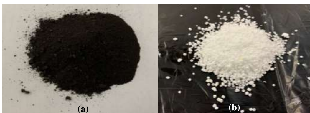
Figure 3.1: Asphalt Modifiers (a) Gilsonite and (b) SBS
