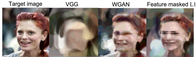
Figure 6.4: Comparison on different rewards. When limited number of strokes are used, both VGG and WGAN yield blurry results. Our feature-masked reward encourages fine details, such as eyes and mouth, be represented at early stage.
