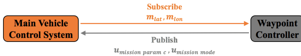
Figure 5-21. Exchange of data between the main vehicle control system and the waypoint controller when the glider changed its target points adaptively.
