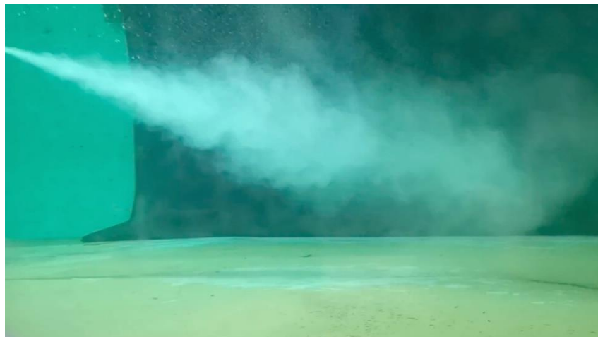
Figure 4-9. Bubble plume generated by the KTM pump in the tow tank.
