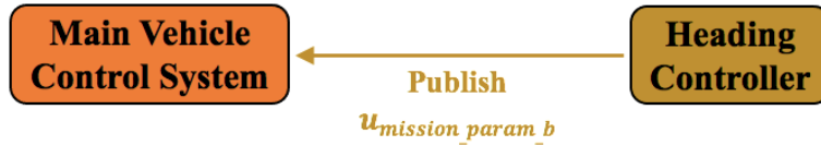
Figure 5-14. Exchange of data between the main vehicle control system and a heading controller when the glider followed a heading commanded by the backseat driver.
