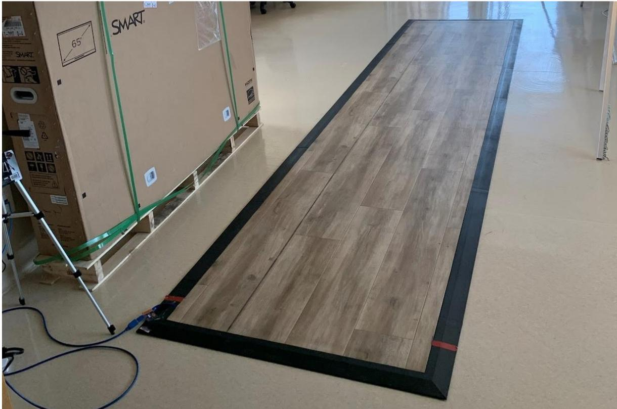
Figure 2.2 GAITRite electronic walkway is embedded with thousands of sensors and attached to the floor.
