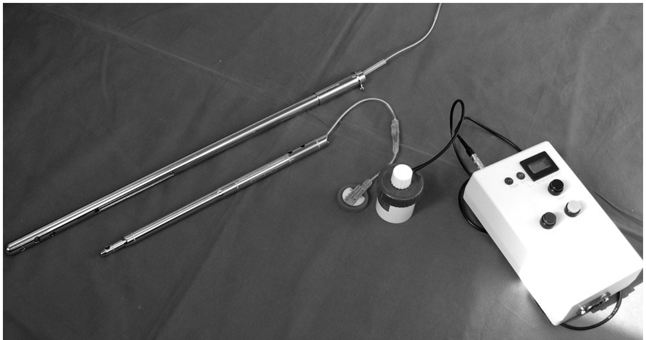
Figure 4.3 Picture of Fitbone Intramedullary Nail and External control device. Transmitter is placed on skin surface over subcutaneously placed receiver [81] . Reprinted with permission Krieg, A.H., et al., Intramedullary leg lengthening with a motorized nail . Acta Orthop, 2011. 82 (3): p. 344-50 DOI: 10.3109/17453674.2011.584209.
