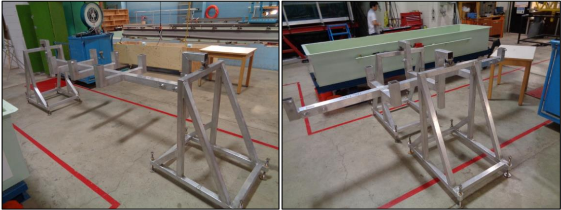
Figure 4.3: Swing frame used to calculate the vertical center of gravity and the mass moment of inertia in the roll (left) and pitch (right) configurations [7].
