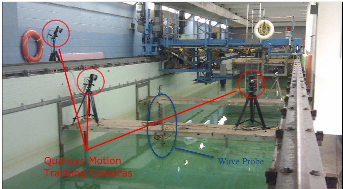
Figure 4.6: Location of the Qualisys motion tracking cameras during the experiment.
