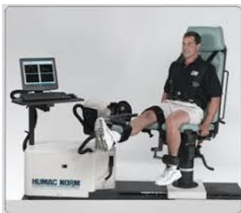
Figure 2: CSMi Humac Norm in Seated Knee Extension/Flexion Position (We opted to change hand position to cross-shoulder position for methodological concerns)
