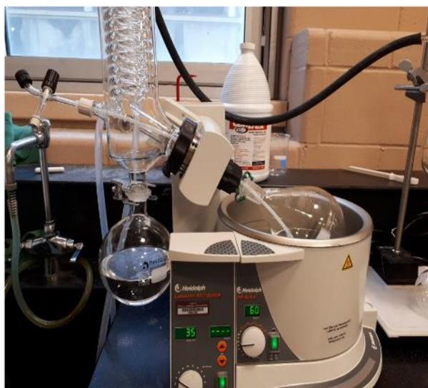
Acetone removed by rotary evaporation
