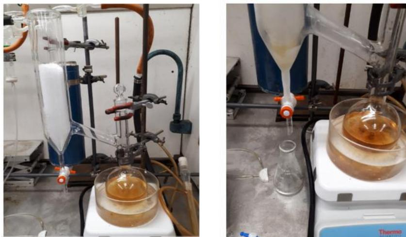
Distillation of used, sulfur-loaded IL in an oil bath at  $110^{\circ}\text{C}$  to remove  $\text{H}_2\text{O}_2$
