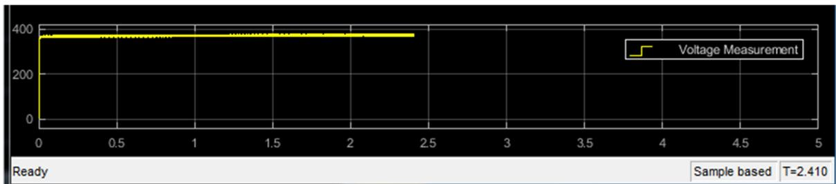
Figure 3. 10: Output voltage from the MPPT.
