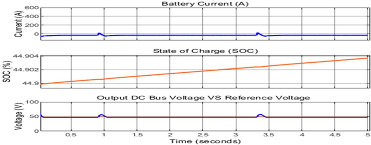
Figure 4. 15: Battery charging current, SOC and output DC voltage due to diesel generator.
