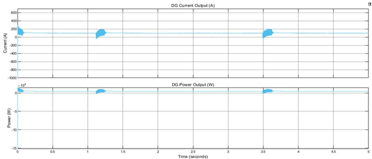
Figure 4.14: Rectified diesel generator output current and power.
