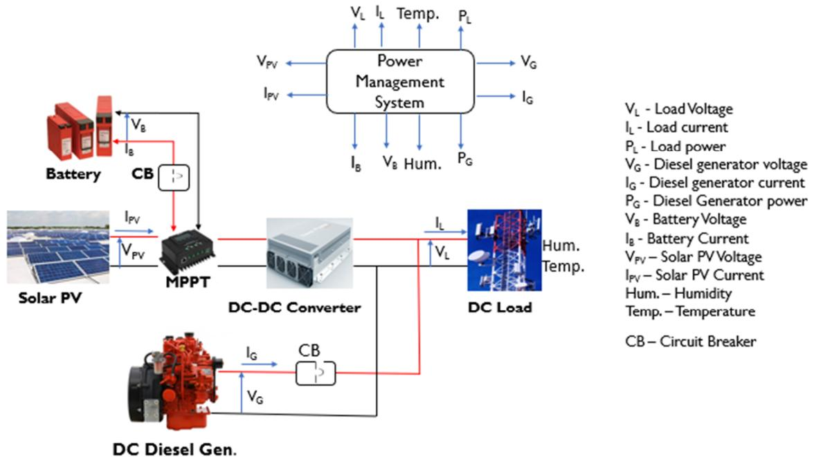
Figure 5. 1: Hybrid power system showing connected devices.
