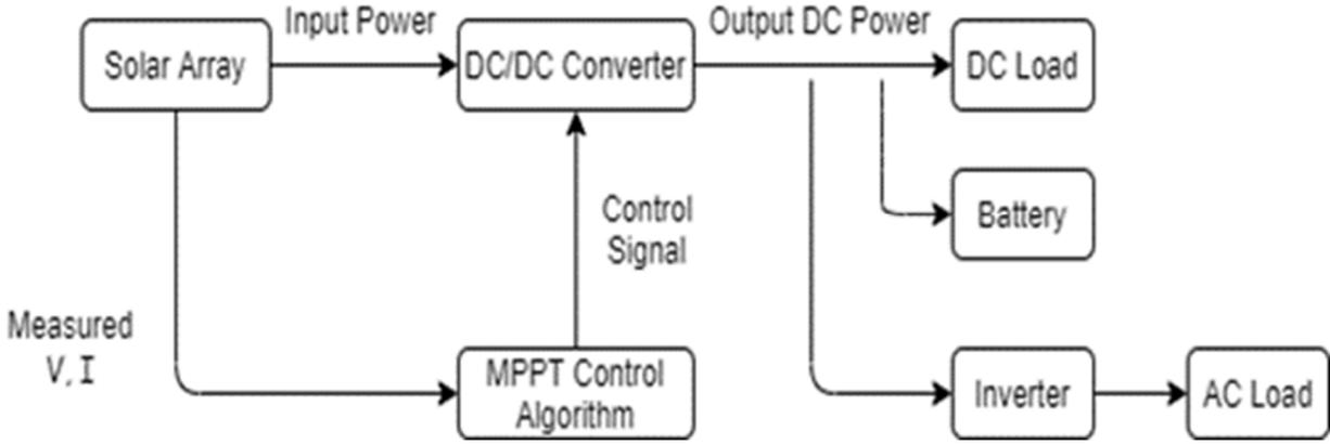
Figure 4. 5: MPPT schematic block.
