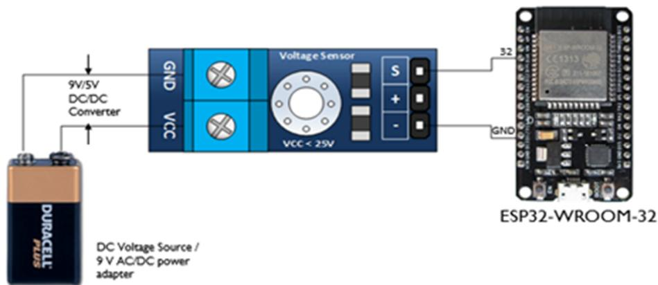
Figure 5. 4: Interfacing diagram of the voltage sensor with ESP32.
