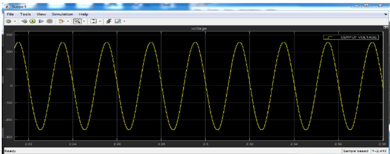
Figure 3. 12: Output voltage from the inverter.
