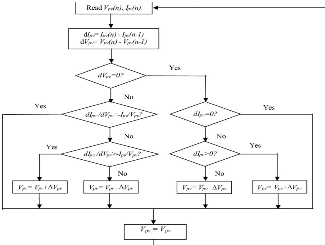
Figure 4. 6: Incremental Conductance algorithm flowchart.
