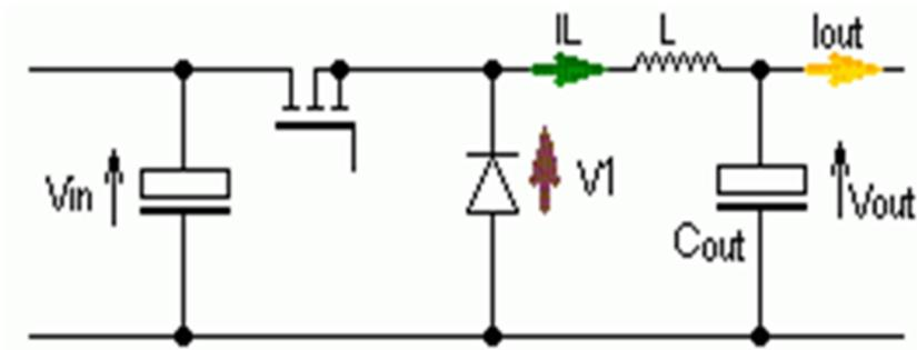
Figure 4. 7: Buck Converter Circuit.
