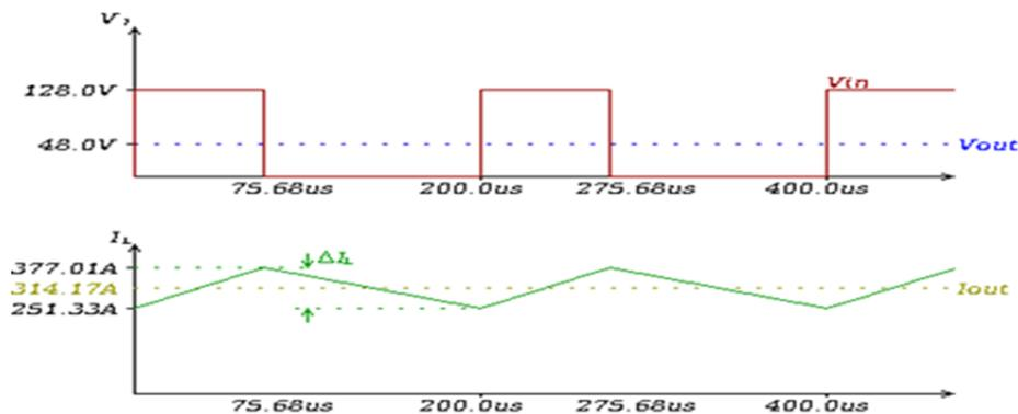
Figure 4. 8: Output Voltage and Current responses of the Buck Converter at MPP Voltage.
