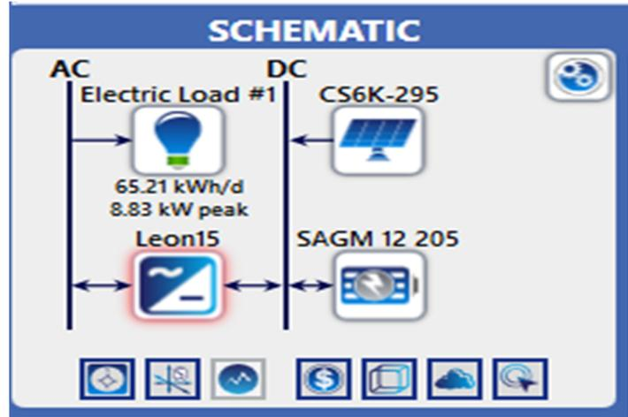
Figure 3. 6: Structure of the system showing the subblocks in HOMER pro.
