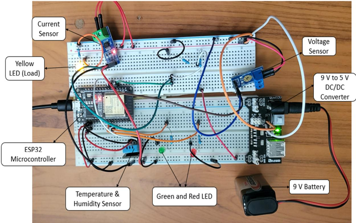
Figure 5. 6: Experimental circuit setup for the IoT SCADA system prototype.
