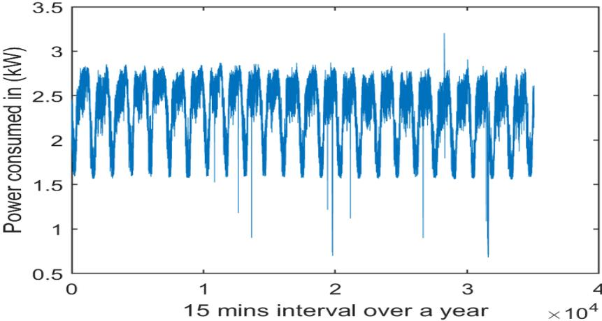
Figure 2.3: Measured load from the rectifier for 1 year.
