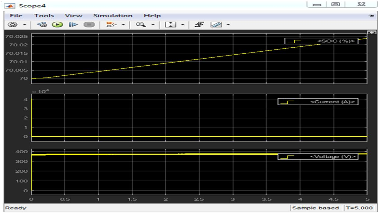
Figure 3. 11: SOC, Current, and Voltage of the battery.
