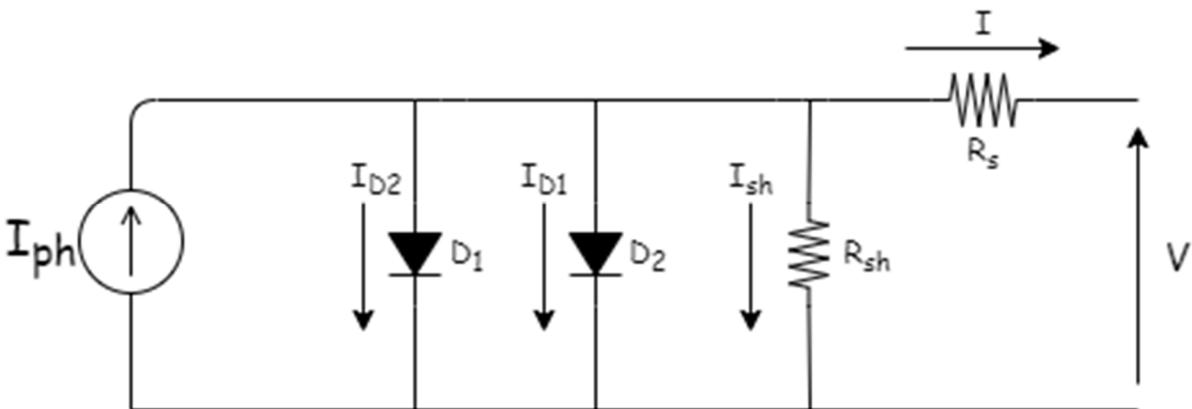
Figure 4. 4: Two-diode solar PV equivalent circuit model
