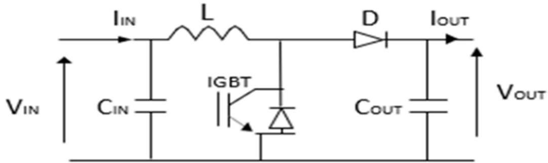
Figure 3. 7: DC-DC boost converter Circuit diagram
