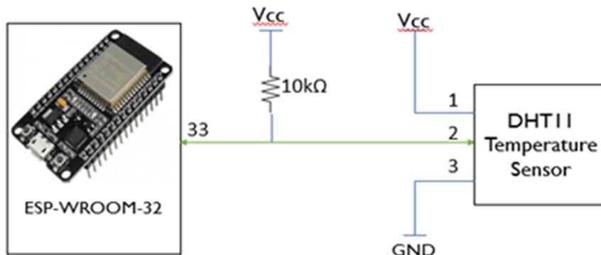
Figure 5. 3: The connection between ESP32 and DHT11.
