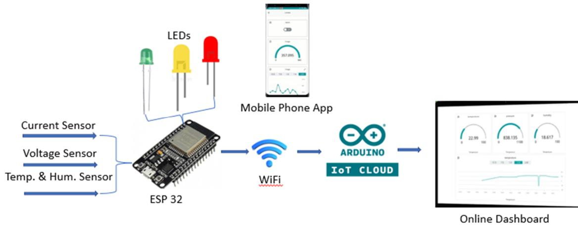
Figure 5. 2: Schematic of the Proposed IoT SCADA system.
