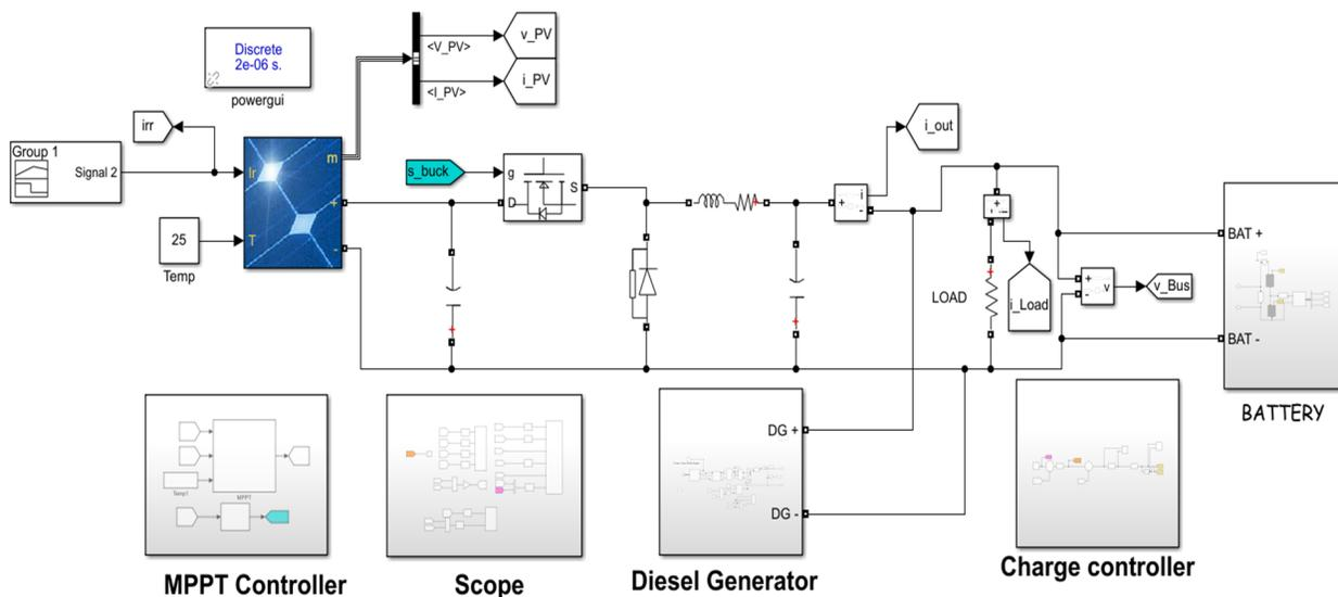
Figure 4. 3: Model of the hybrid system in Simulink.
