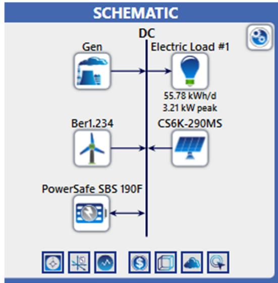
Figure 4. 1: HOMER pro schematic model of the hybrid system units.
