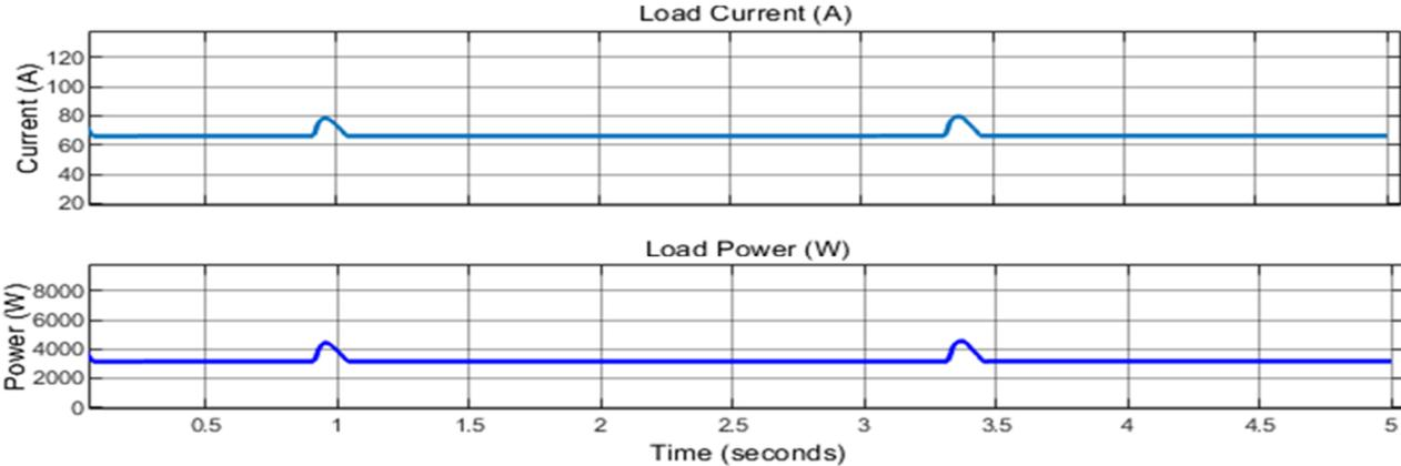
Figure 4. 16: Output current and power due to diesel generator.
