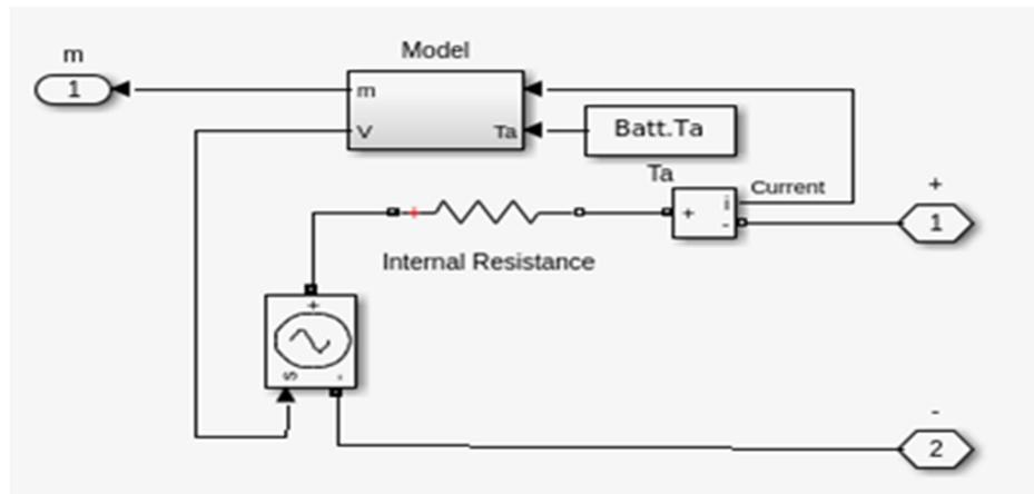
Figure 4. 9: Masked Battery model in Simulink.
