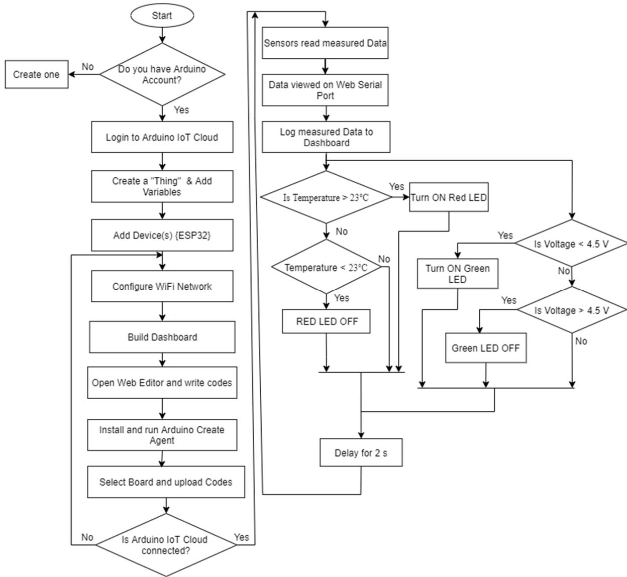
Figure 5. 7: Flowchart of the IoT SCADA system solution.
