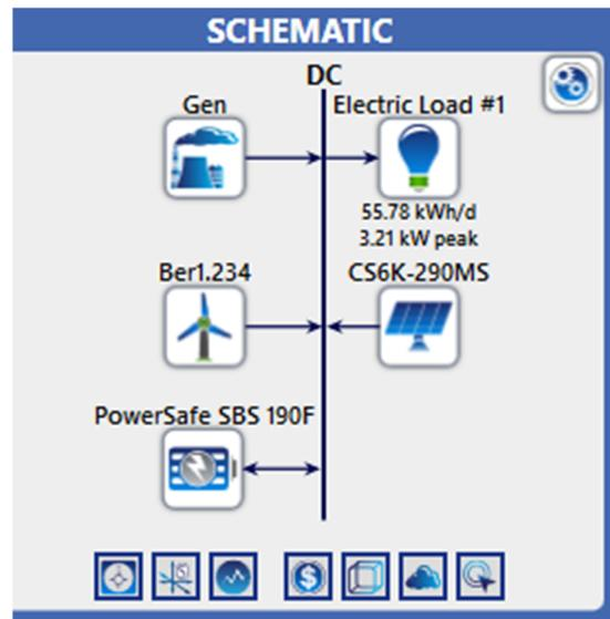
Figure 2. 4: Proposed HOMER schematic model for the Hybrid System.
