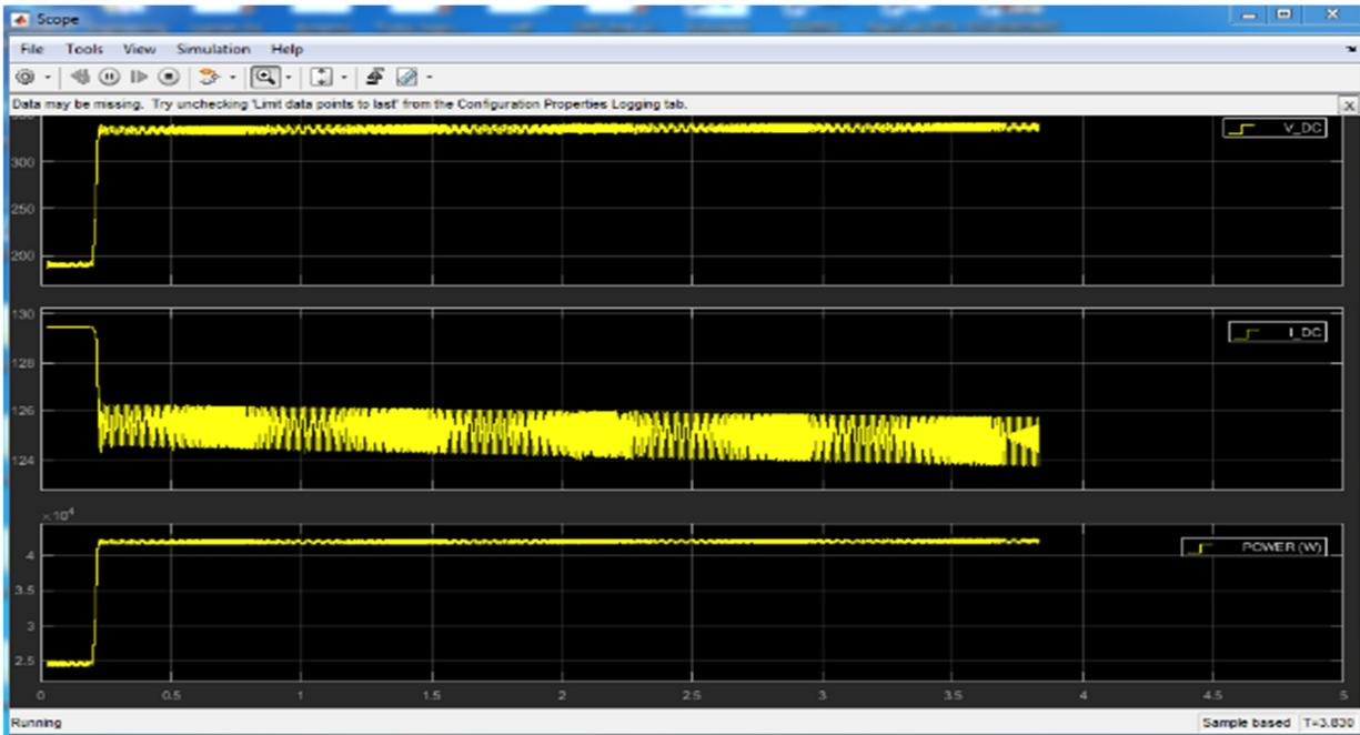
Figure 3. 9: Voltage, Current and Power output from the Solar PV.
