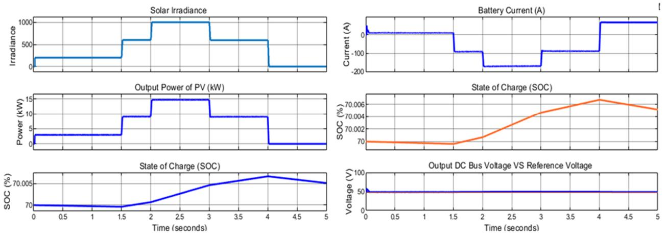
(a) Solar Irradiance, PV output power and SOC of battery.
