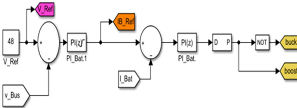
Figure 4. 10: Charge controller topology for the Battery.
