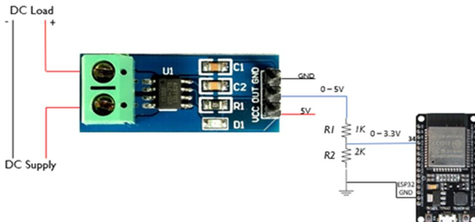
Figure 5. 5: ACS712 connection to ESP32 microcontroller.
