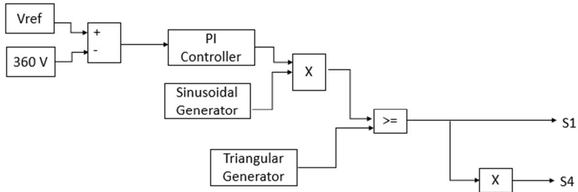
Figure 3. 8: Voltage Controller block for inverter.
