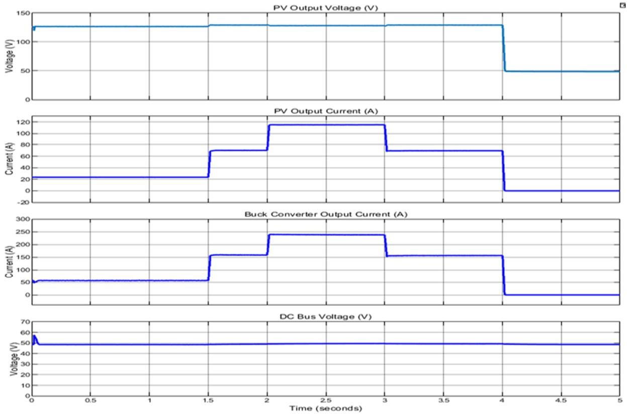
Figure 4. 11: PV voltage, Current, buck converter current and DC bus voltage.
