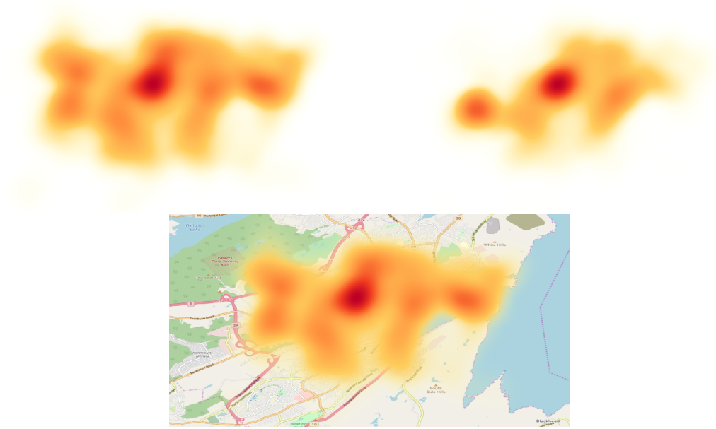
Figure 3.3: Comparison between the original graph (top left), the reduced graph (top right), and the complete interpolated centrality after reduction and reconstruction (bottom). Heat maps represent road scores for downtown St. John's and are closely similar, albeit one generated through reduction and reconstruction. (Generated by QGIS [98])
