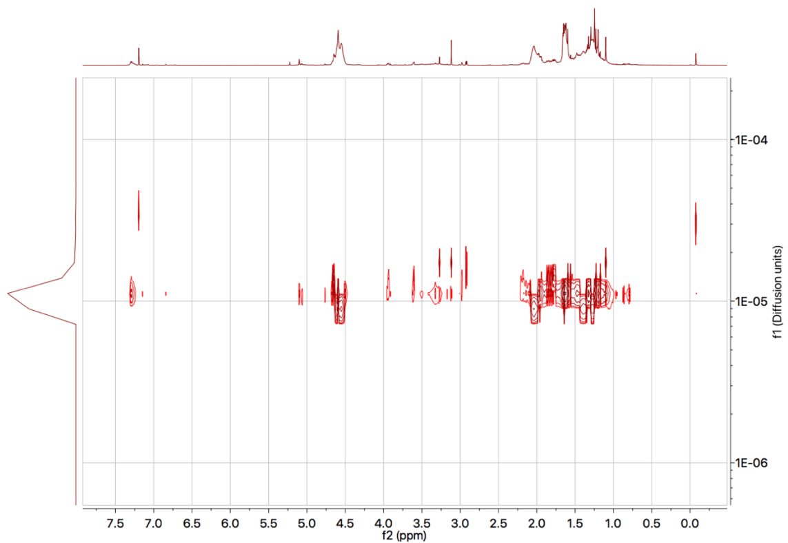
Fig. 2.5: DOSY spectrum of poly(cyclohexene oxide) and poly(cyclohexene carbonate) synthesized via 30 min of homopolymerization prior to CO 2 pressurization (40 bar), showing two or more distinct polymer products. Poly(cyclohexene oxide) -5.99 \log(\text{cm}^2 \text{s}^{-1}) , poly(cyclohexene carbonate) -6.49 \log(\text{cm}^2 \text{s}^{-1}) , CDCl 3 , CHO & CH 2 Cl 2 -4.66 \log(\text{cm}^2 \text{s}^{-1}) . (500 MHz, CDCl 3 , 298K)
