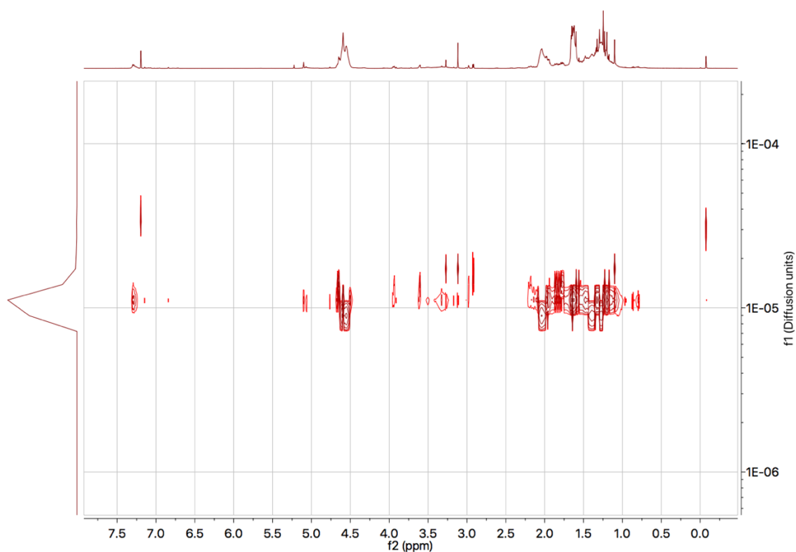
Fig. 2.4: DOSY spectrum for LO/CHO copolymer. Polymer -5.05 to -4.95 \log(\text{cm}^2 \text{s}^{-1}) , \text{CDCl}_3 -4.56 \log(\text{cm}^2 \text{s}^{-1}) , CHO -4.66 \log(\text{cm}^2 \text{s}^{-1}) . (500 MHz, \text{CDCl}_3 , 298K)
