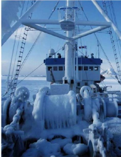
Figure 3-5 Extreme Marine Icing Scenario (Cammaert, 2013)
