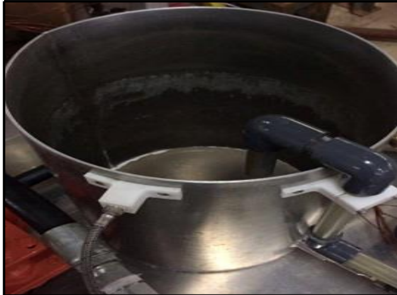
Figure 3.4 Tank of the Experimental Flow Loop Pipeline.
