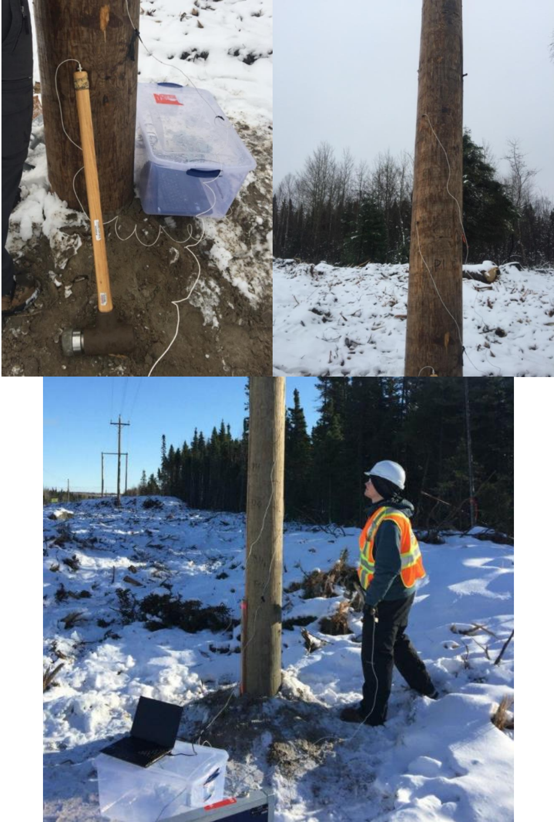
Figure B.1: Field modal test a) Modal hammer b) Accelerometers c) Test setup
