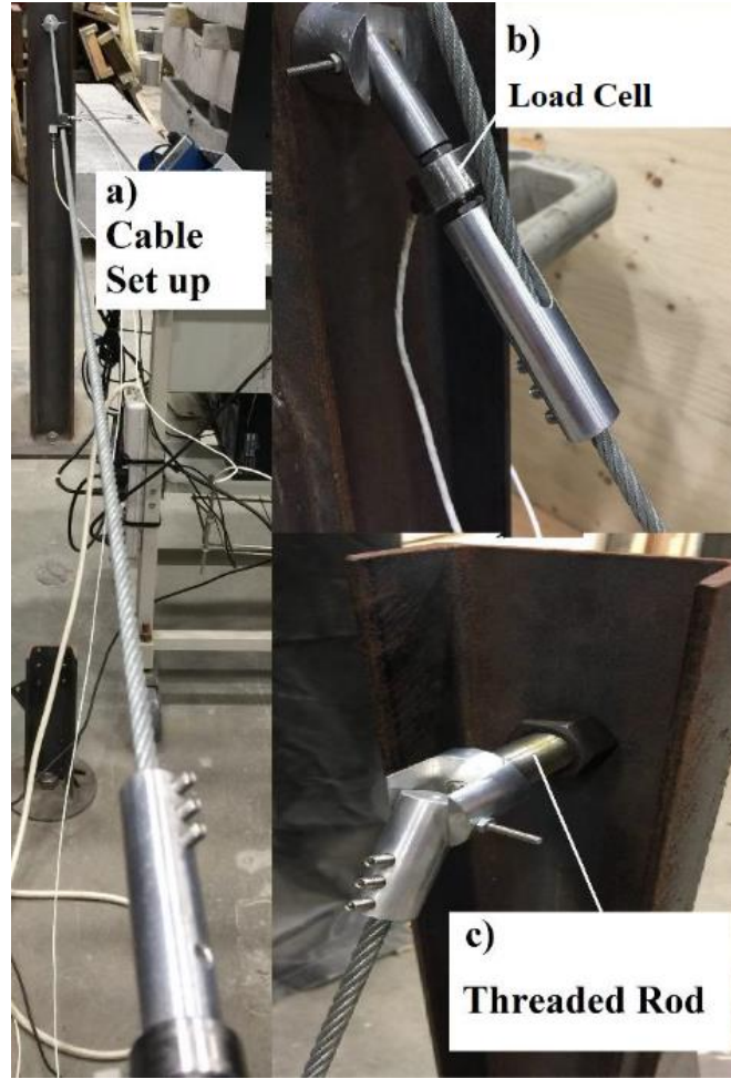
Figure 6.16: Cable vibration test set up a) Test set up b) In-line load cell c) Threaded rod
