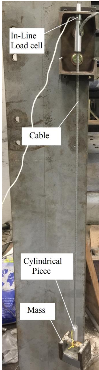
Figure 6.13: Axial stiffness and damping measurement set up
