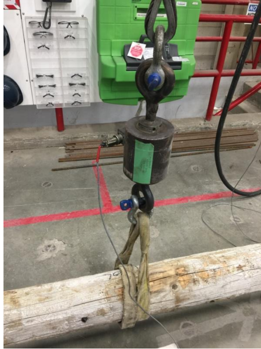
Figure A.3: Load cell used to measure the applied load
