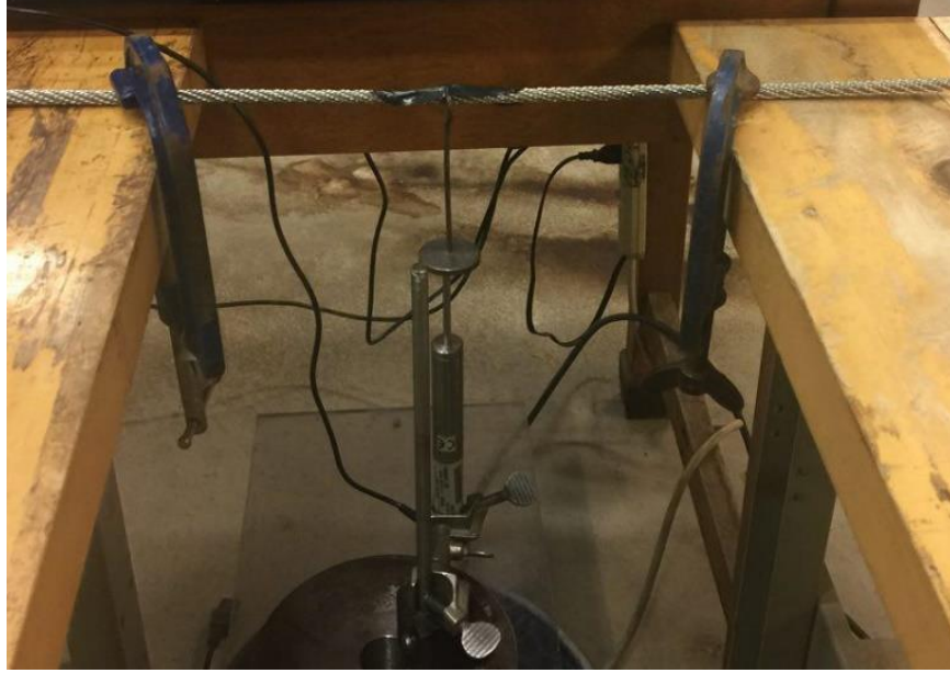
Figure 4.4: Setup for Bending Stiffness Measurement
