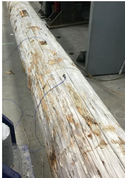
Figure B.6: Accelerometers mounted on the pole in the lab
