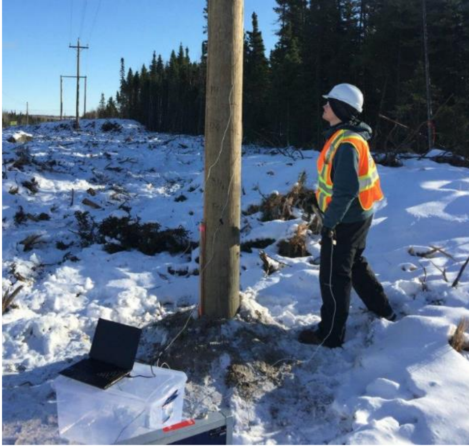
Figure 1.3: Field modal test in Goose bay, Labrador
