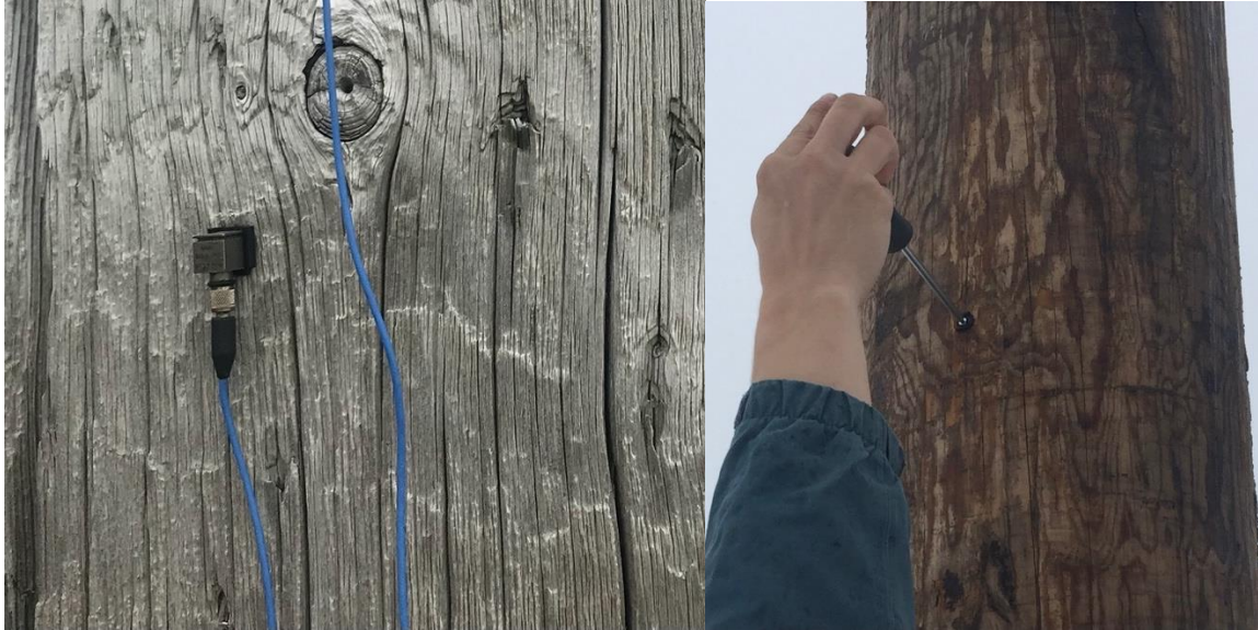
Figure B.2: Mounting accelerometer a) accelerometer in the rubber piece b) bolting the piece to the wooden pole
