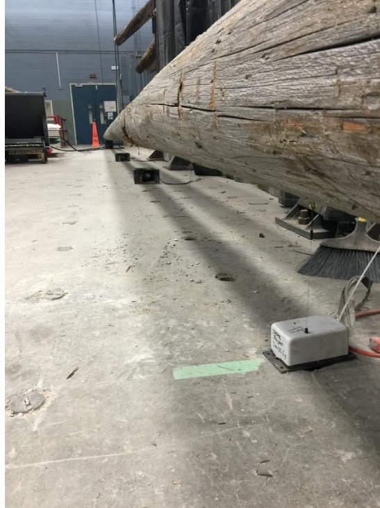
Figure A.4: Measurement of displacement in four different positions along the pole
