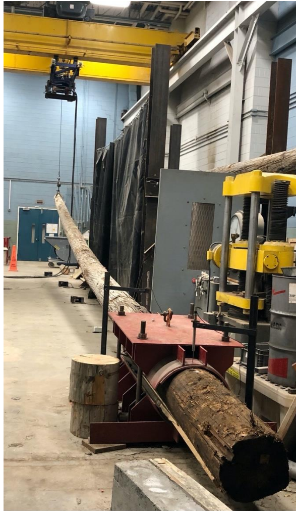
Figure A.1: Destructive test of full-scale pole
