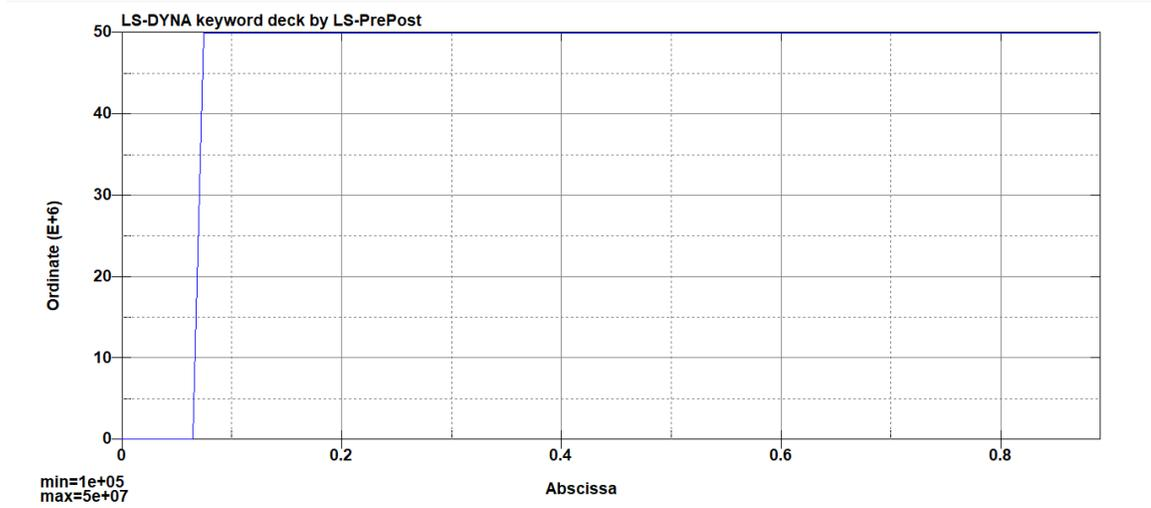
Figure 17 - Crushable Foam Material Model Stress-Strain Load Curve
