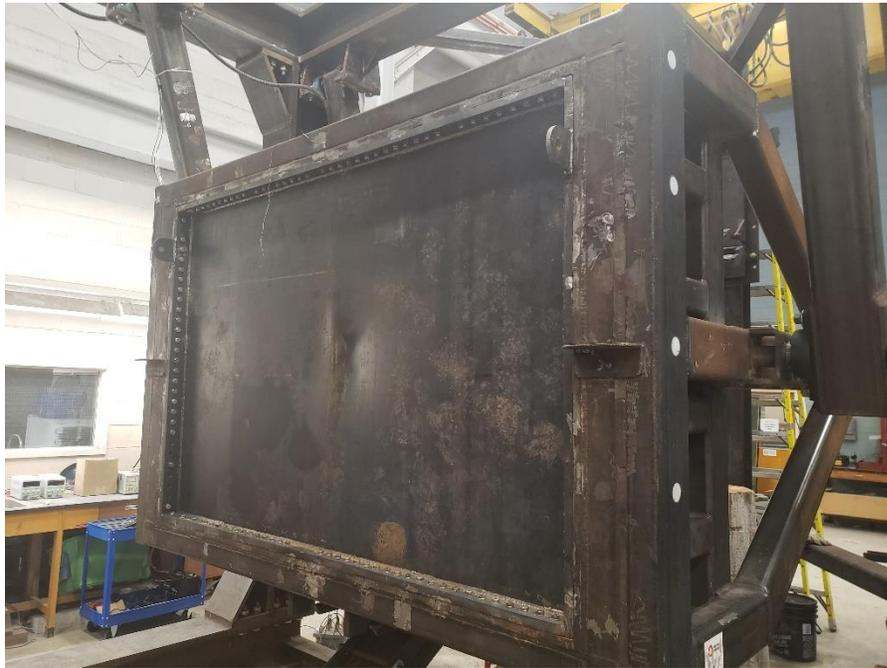
Figure 4 - LPA Grillage Holding Carriage
