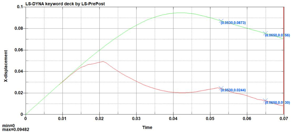
Figure 27 - Original Ex-HMCS IROQUOIS Panel FEA Maximum Displacement
