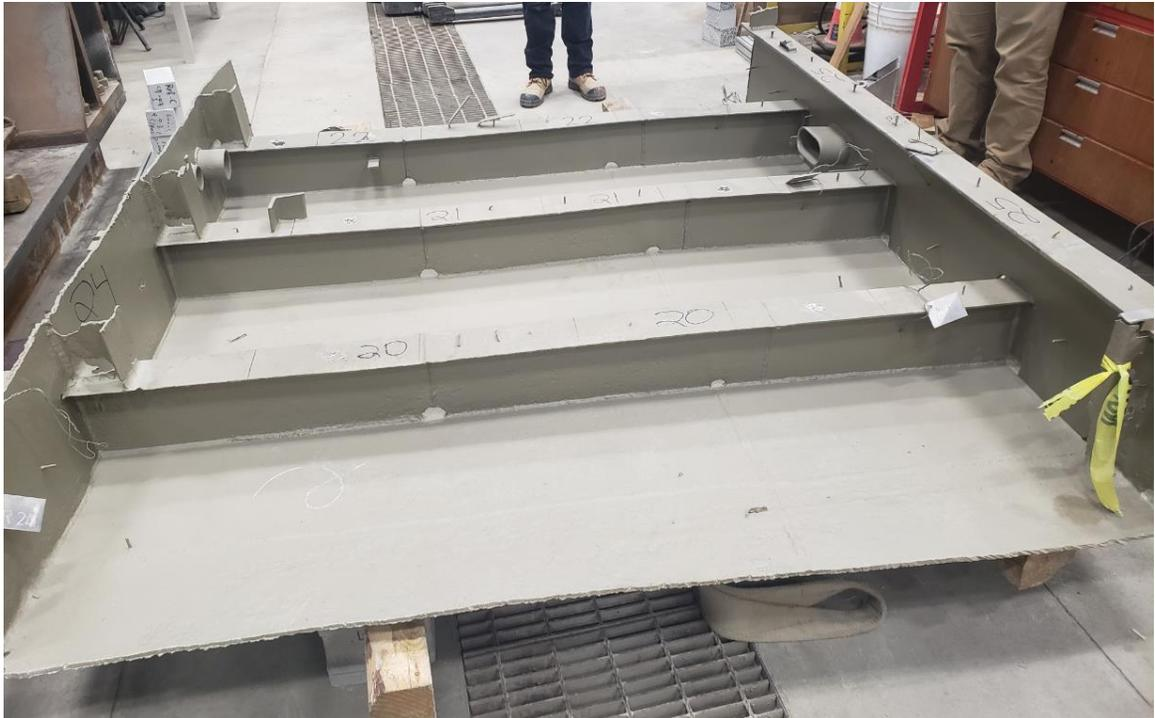
Figure 2 – One of the Six HMCS IROQUOIS Grillages, Intact
