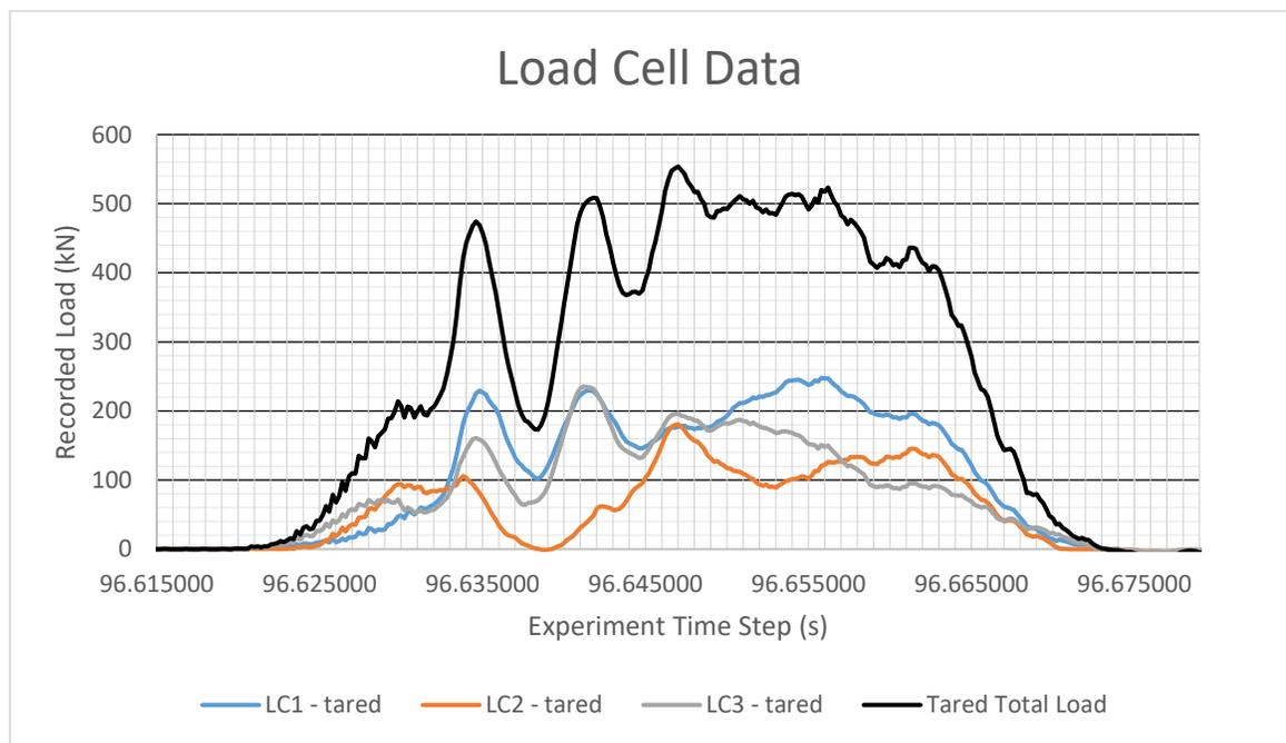
Figure 24 - Original Ex-HMCS IROQUOIS Panel Load Cell Data (Figure was generated by S. Andrade, and is used with permission)
