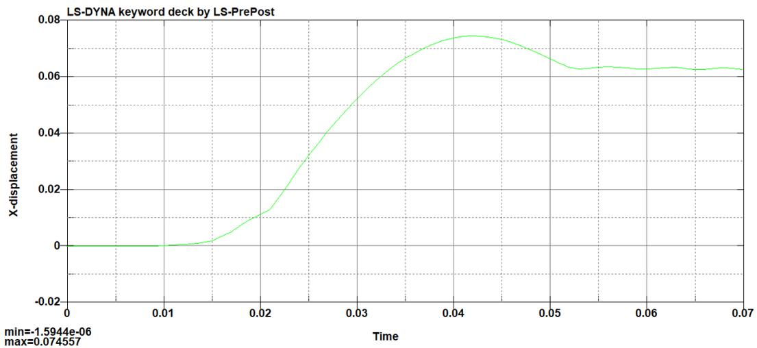
Figure 28 - Dent Depth versus Time of Original Grillage
