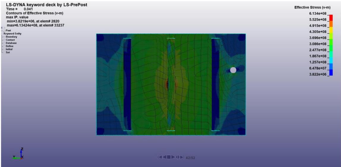
Figure 31 - Original Ex-HMCS IROQUOIS Panel Von Mises Stress - Back
