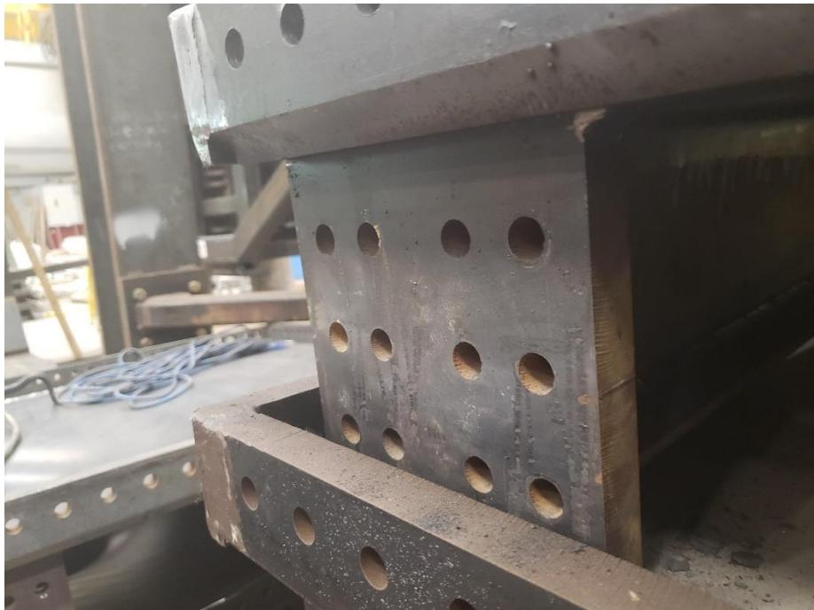
Figure 6 - Grillage Stiffener Boundary Connectors
