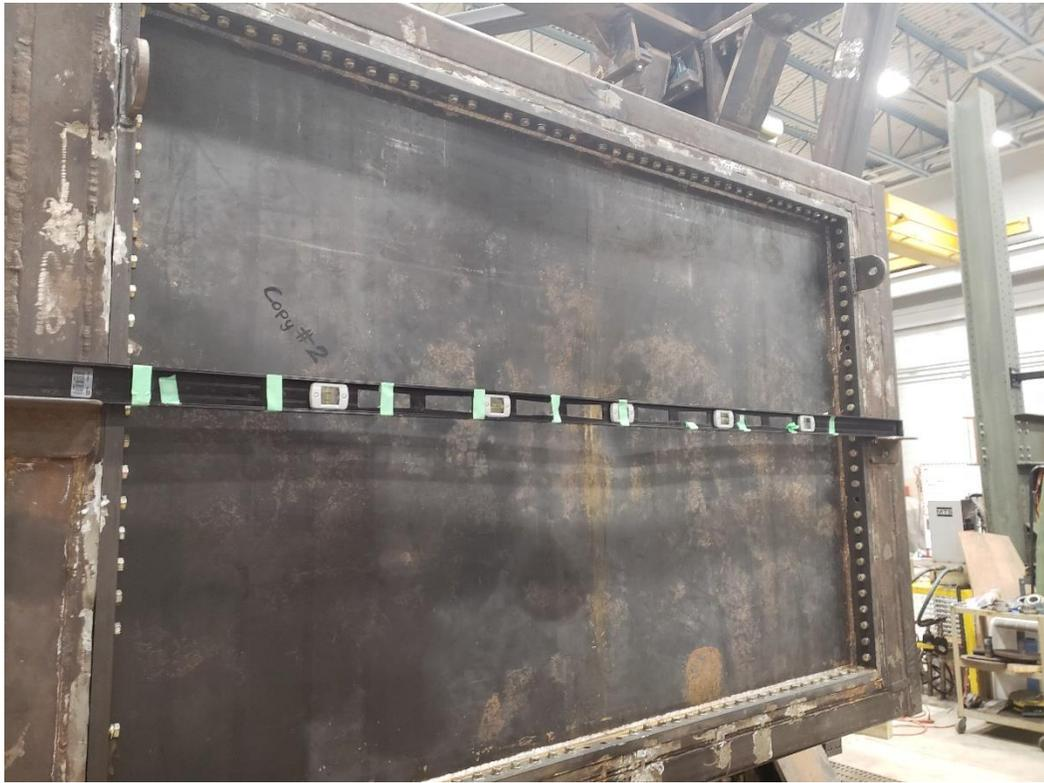
Figure 22 - Experiment Displacement Data Point Locations
