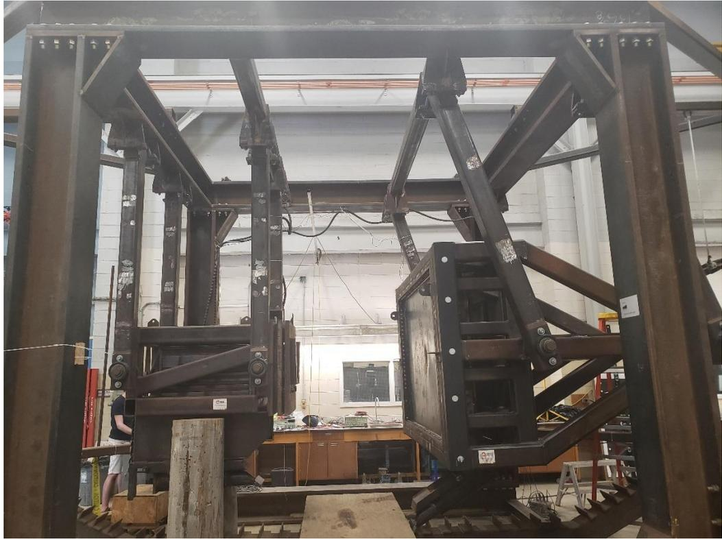
Figure 3 - Large Double-Pendulum Apparatus
