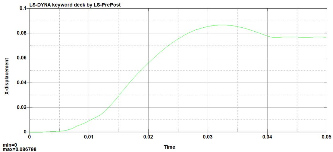
Figure 34 - Dent Depth versus Time of Copy Grillage
