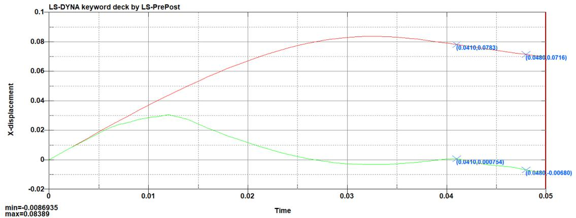
Figure 33 - Original Ex-HMCS IROQUOIS Panel FEA Maximum Displacement
