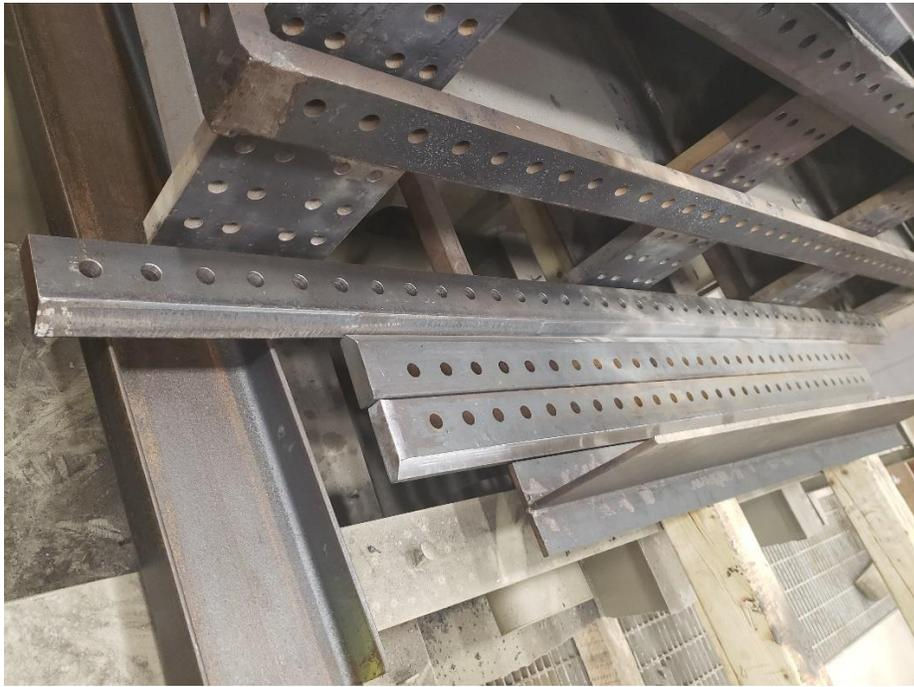
Figure 5 - Grillage Plating Boundary Connectors
