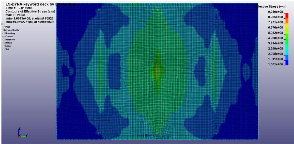
Figure 36 - Copy Ex-HMCS IROQUOIS Panel Von Mises Stress - Front
