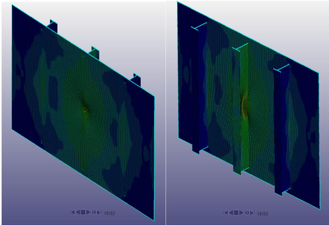
Figure 38 - Copy Ex-HMCS IROQUOIS Panel Von Mises Stress - Isometric Front and Back
