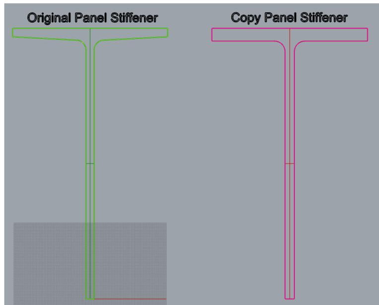
Figure 11 - Stiffener Cross-Sections
