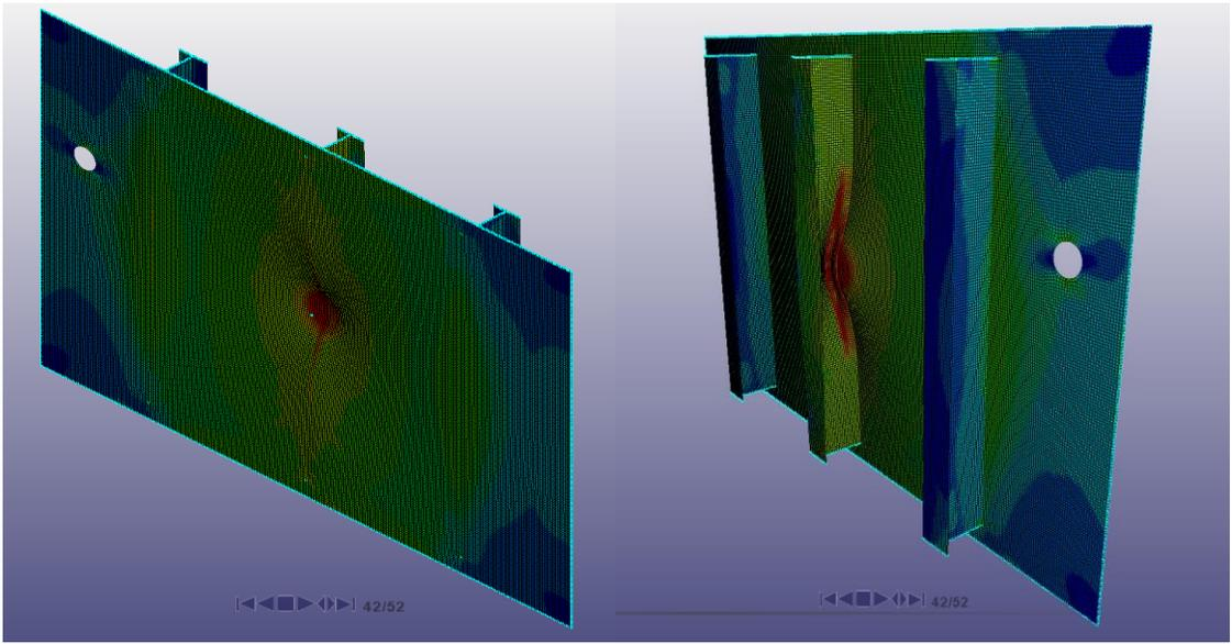
Figure 32 - Original Ex-HMCS IROQUOIS Panel Von Mises Stress - Isometric Front and Back
