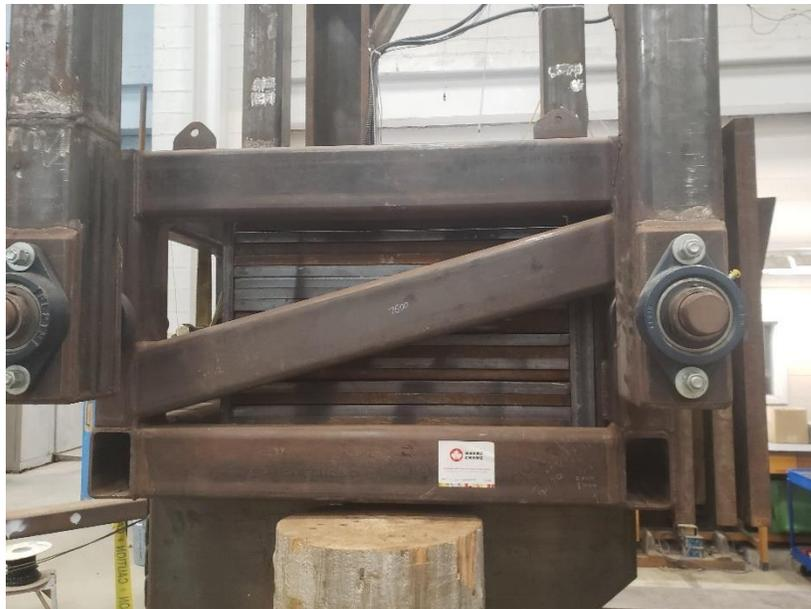
Figure 9 - Ice Indenter Carriage Additional Weight
