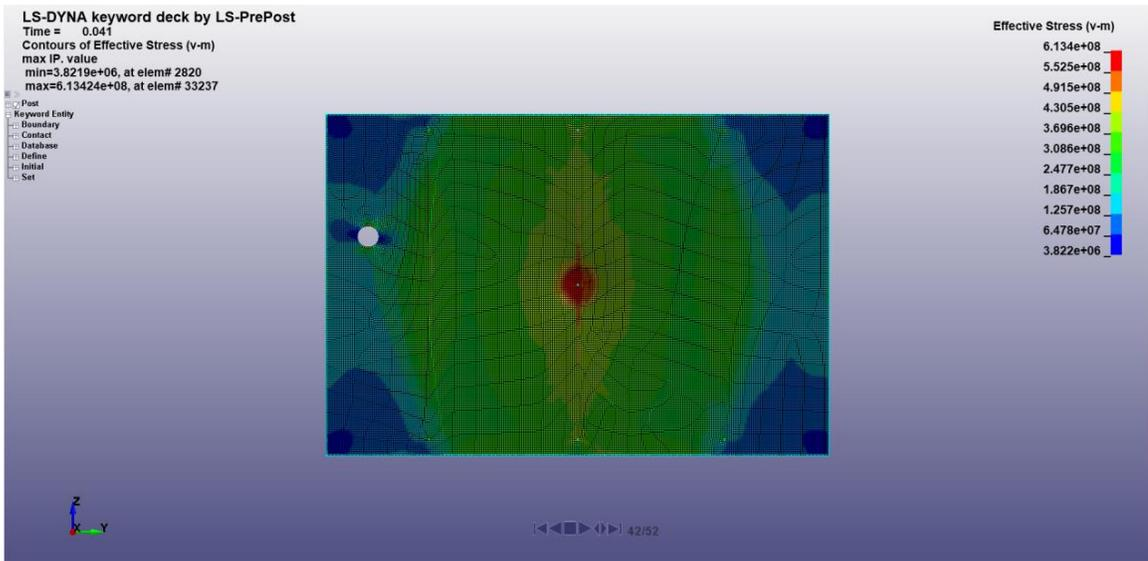
Figure 30 - Original Ex-HMCS IROQUOIS Panel Von Mises Stress - Front
