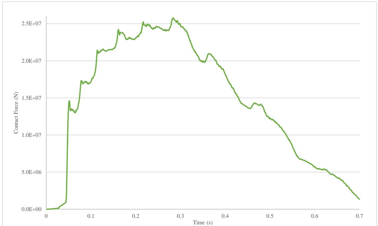
Figure 6-40 Contact force for ice collision with long cylinder shape (3000-tonne bergy bit)
