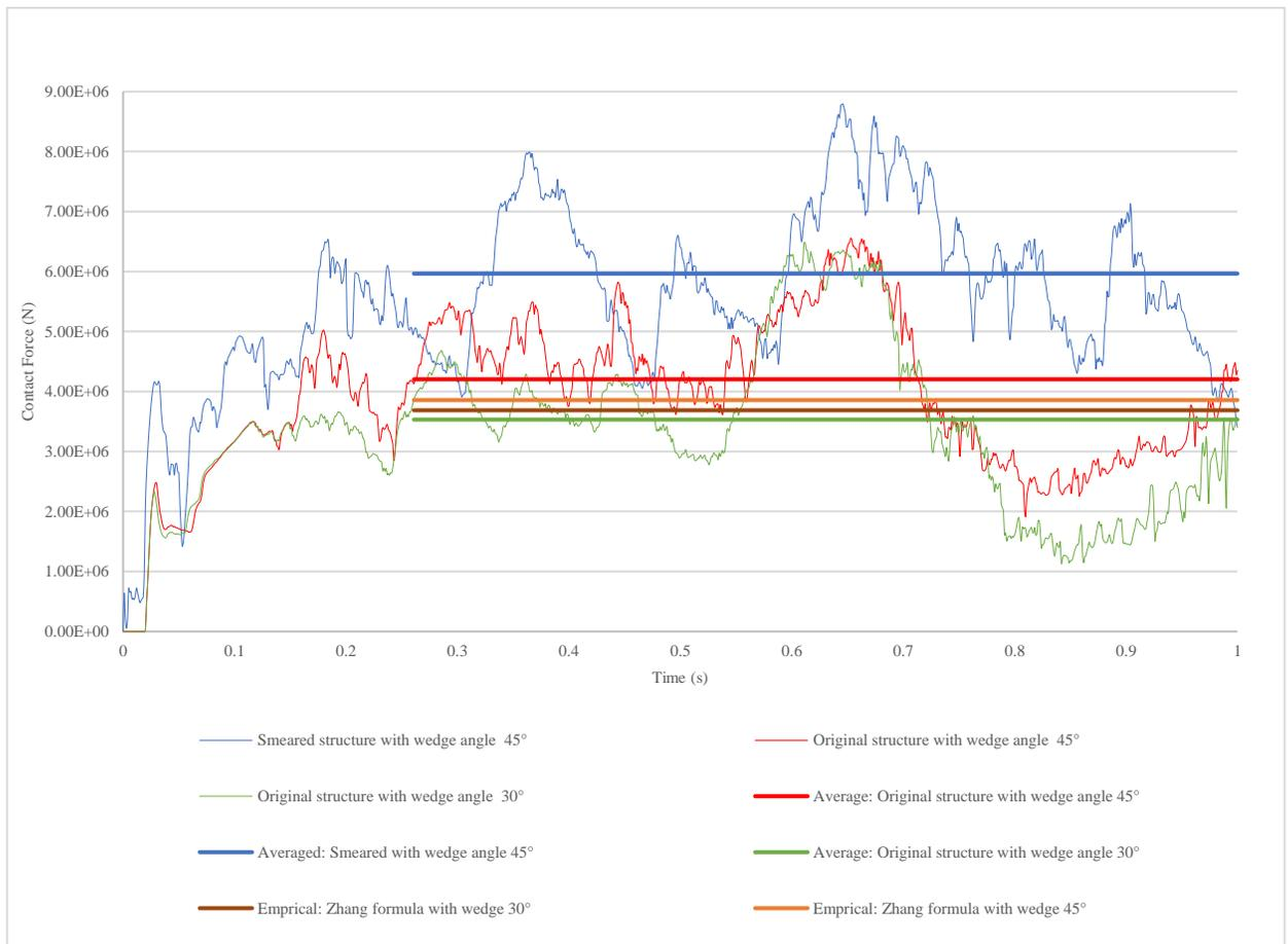
Figure 8-8 Contact force for various simulated wedge cutting
