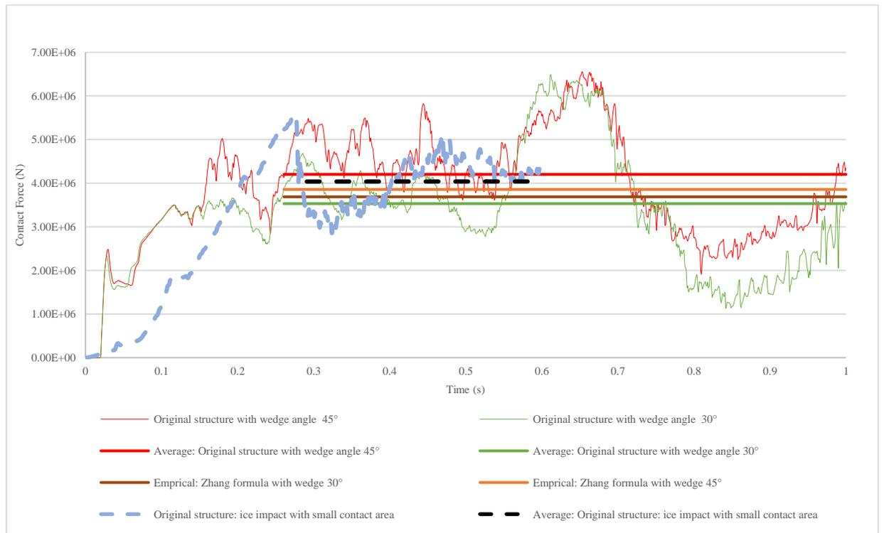
Figure 8-9 comparisons of contact force in wedge cutting and ice impact with the small contact area
