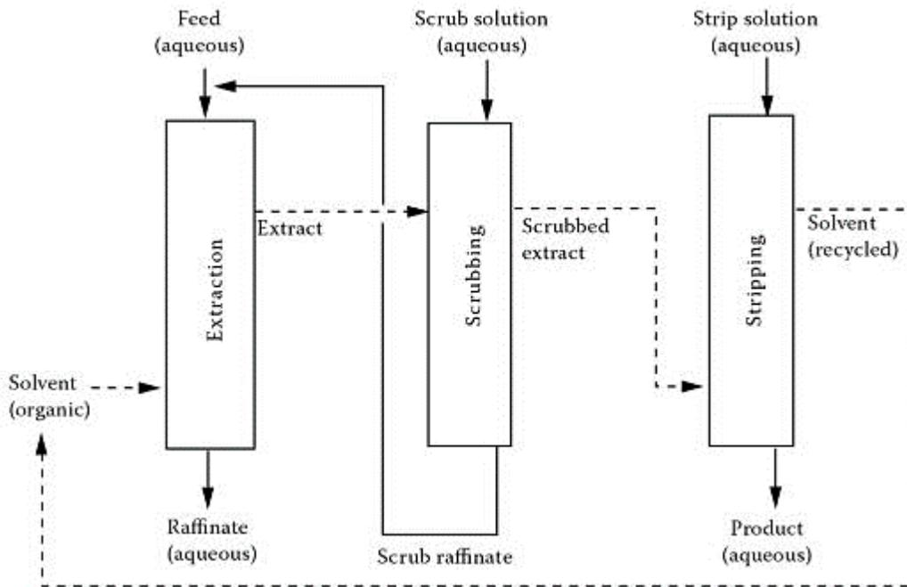
**Figure 1.** The schematic diagram of the solvent extraction process
