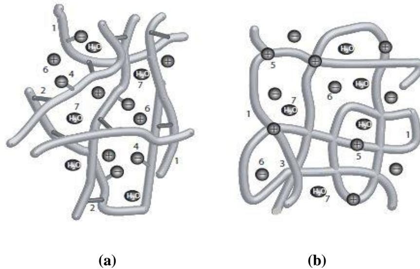
**Figure 3.** Schematic representation of polymeric cross-linked ion exchanger. (a) Cross-linked cation exchange material; (b) Unrecognisable cross linked anion exchange materials. 1 – Polymeric chain; 2 – cross-link; 3 – physical knot; 4 – negatively charged cation exchange group linked with the chain; 5– positively charged anion group attached to the chain; 6 – counterion; 7 – water (Zagorodni, 2006).
