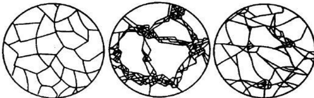
**Figure 2.** Structures of gel type, macroporous and isoporous ion exchangers (left to right) (Dorfner, 2011)
