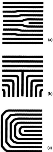
Figure 4.10: An example of a dislocation (a) and examples of the two types of disclinations which can occur in the stripe phases (b) and (c). These examples are schematics. Black regions have magnetic moments along the positive \hat{z} direction, while white regions have magnetic moments along the -\hat{z} direction.
