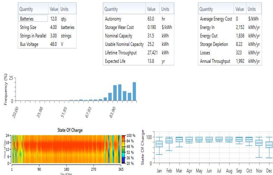
Figure 3.12. Results for the utilized battery bank of the proposed PV-battery system
