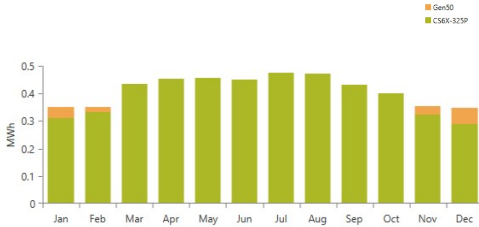
Figure 4.4. Electrical simulation results for the hybrid PV-Gen-Batt system
