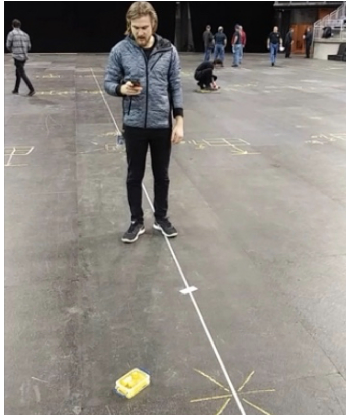
Figure 5: Christian examining the disto at the centre line
