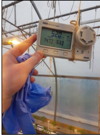
Figure 6 HOBOTM data logger suspended in experimental greenhouse. Used to collect ambient air temperature, CO 2 concentration, and relative humidity levels within the greenhouse.
