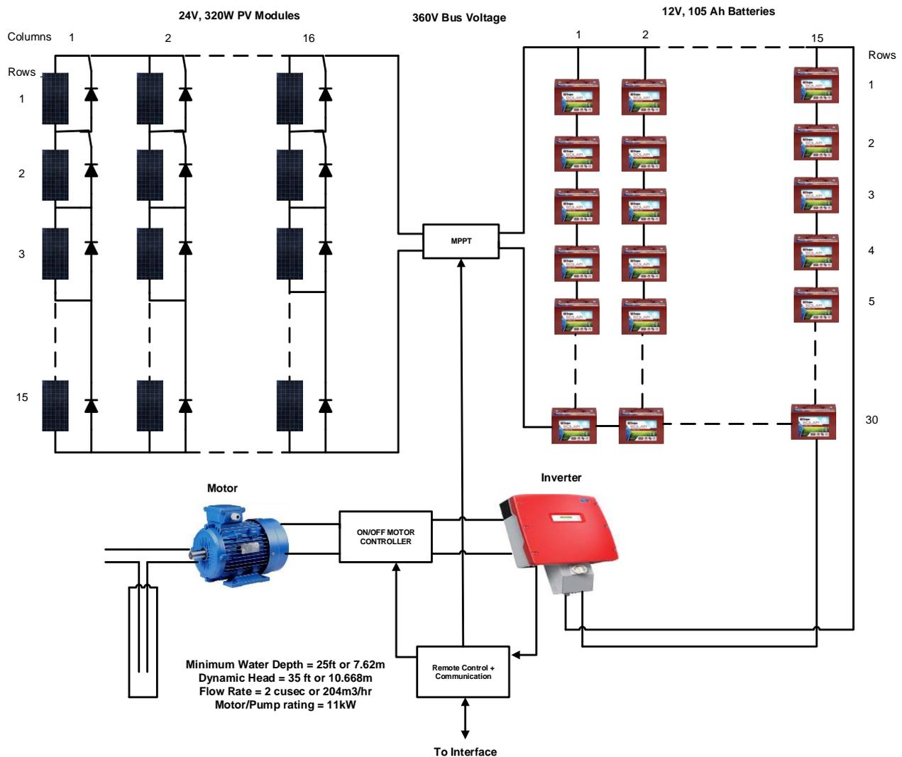
**Figure 20:** Overall proposed solar water pumping system with a battery bank.
