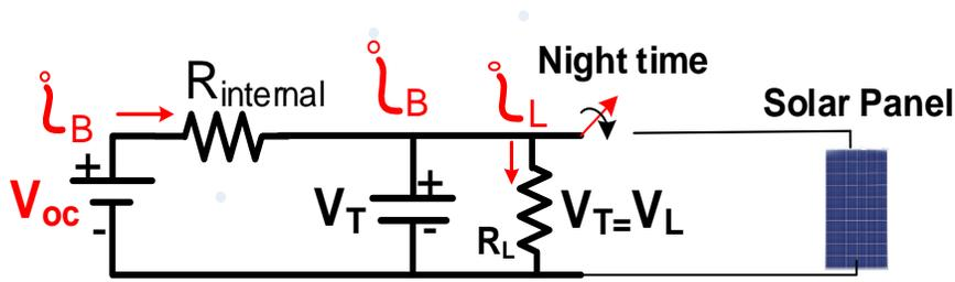
Figure 33: Battery feeding the load
