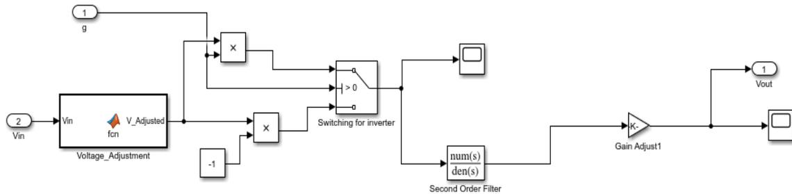
Figure 38: Inverter model in MATLAB/Simulink
