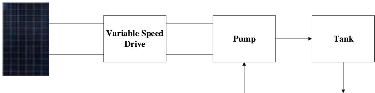
Figure 3: Solar water pumping system with water tank storage
