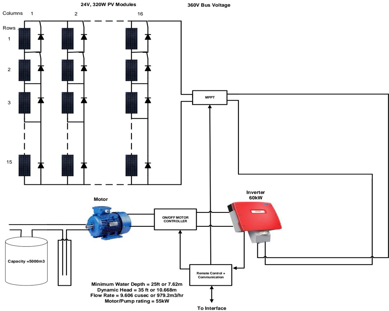
Figure 52: Proposed solar water pumping system with water tank.
