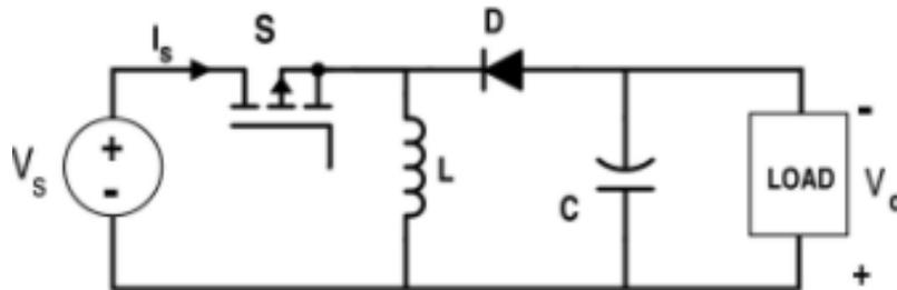
Figure 8: A Buck-Boost Converter [15]
