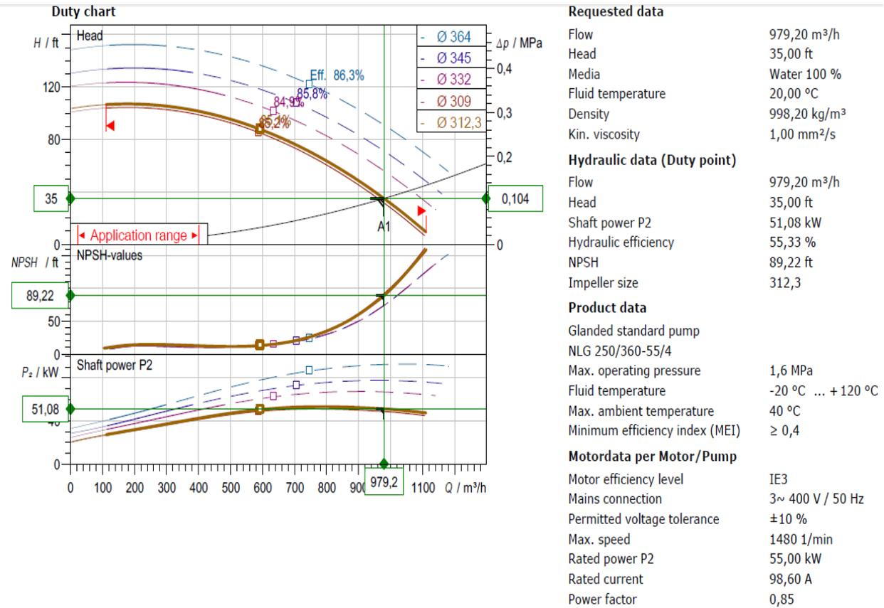
Figure 47: Parameters that led to the motor/pump selection.
