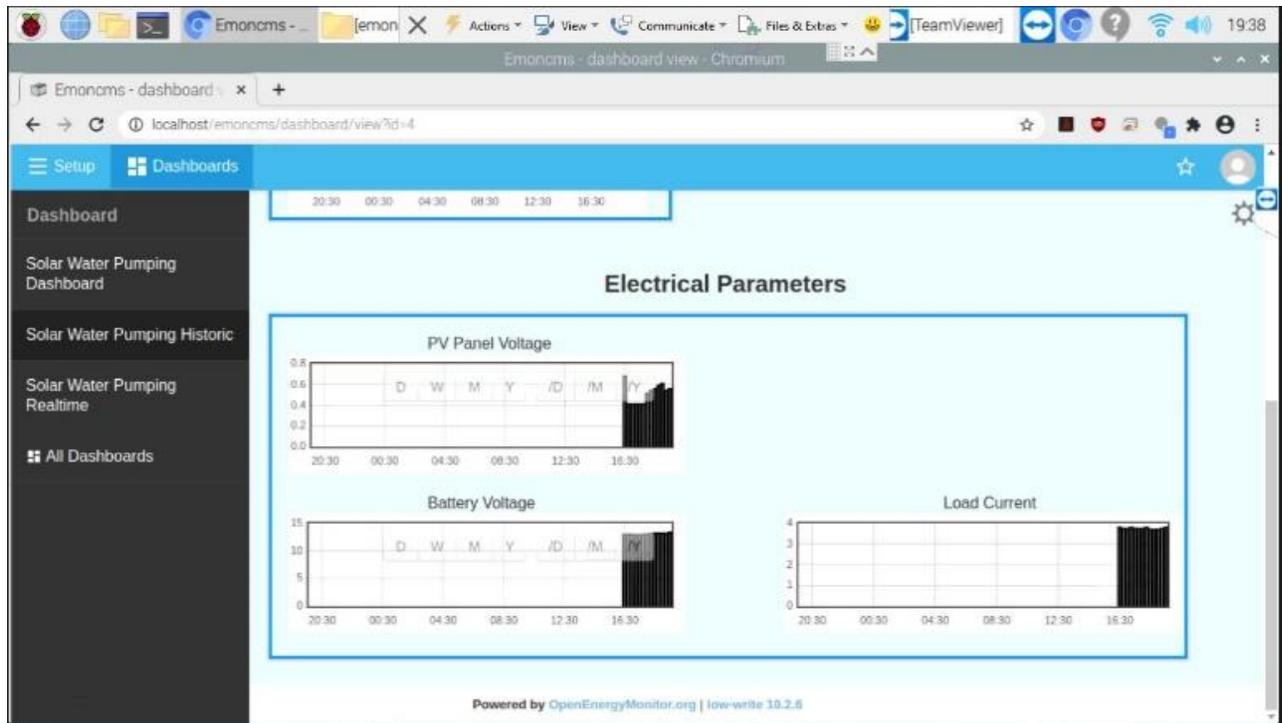
Figure 66: Historic or logged data in Emoncms for a solar water pumping system (Electrical Parameters)
