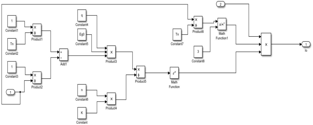
Figure 27: Saturation Current Equation modeled in MATLAB/Simulink
