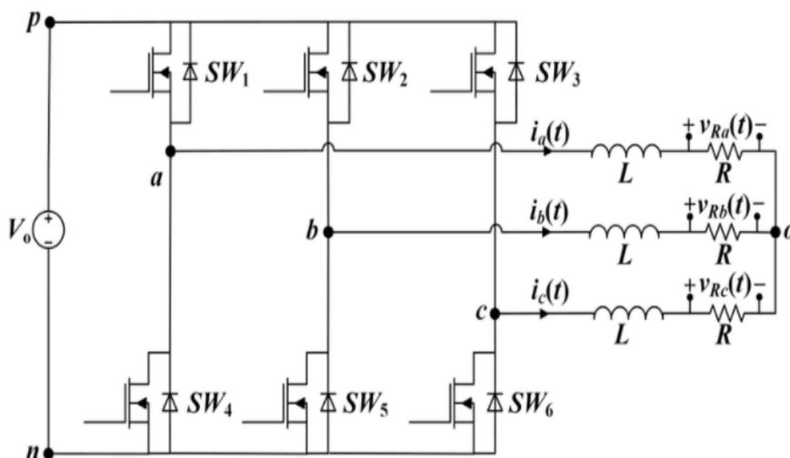
Figure 9: Three Phase Full bridge inverter configuration [16]
