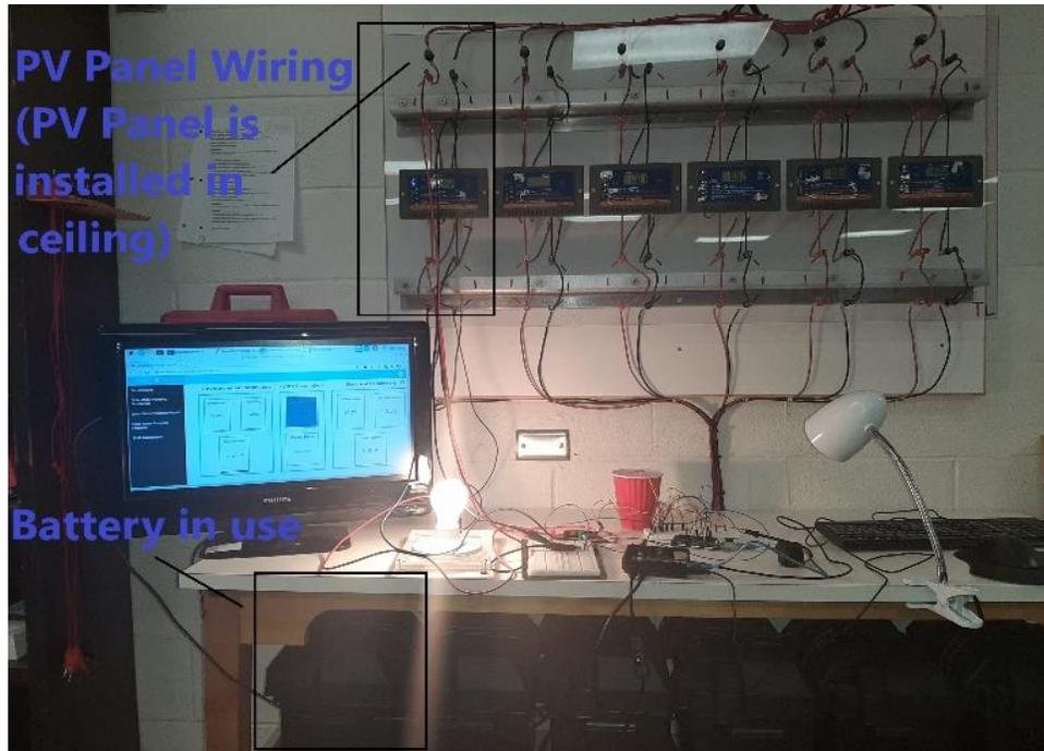
Figure 59: Prototype of Proposed SCADA system in Lab (With Lab setup)
