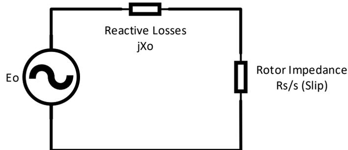
Figure 39: Equivalent model for Inductive Motor
