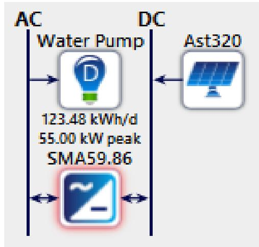
Figure 50: Proposed PV based water pumping system with Water Tank
