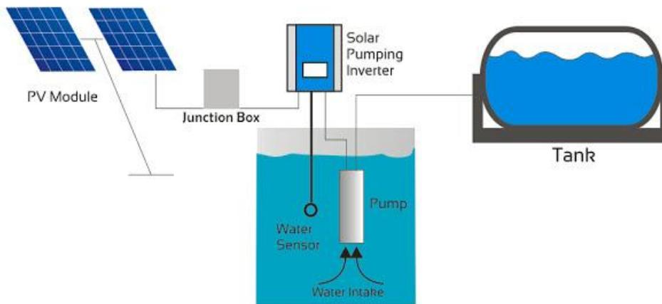
Figure 48: Generic block diagram of solar water pumping with the water tank
