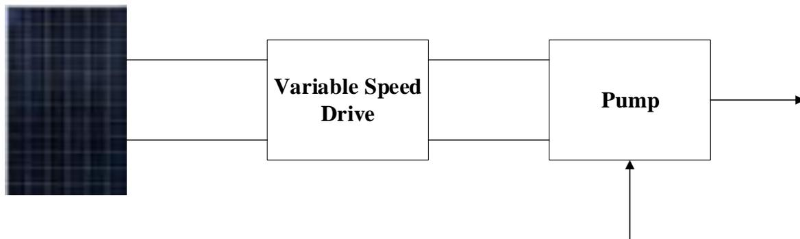
Figure 1: A variable speed drive based solar water pumping system
