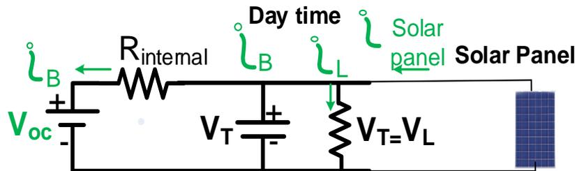
Figure 34: Solar panel feeding the load and battery
