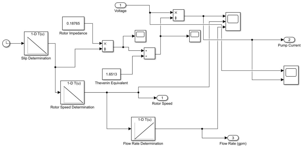
Figure 40: Modeling of Induction Motor in MATLAB/Simulink
