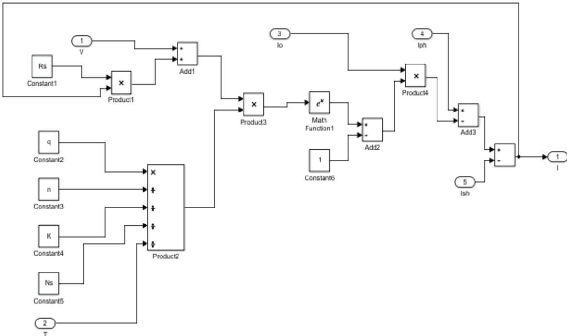
Figure 30: Output PV current modeled in MATLAB/Simulink
