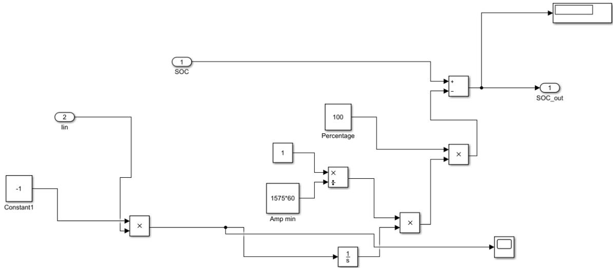
Figure 36: SOC block for modeled battery bank
