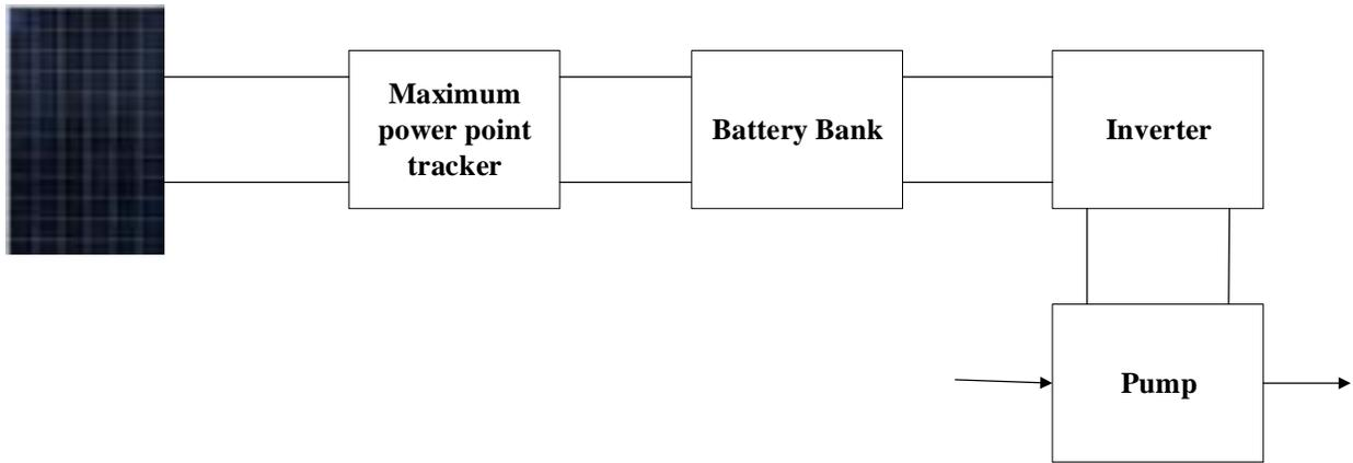
Figure 2: Battery bank based solar water pumping system
