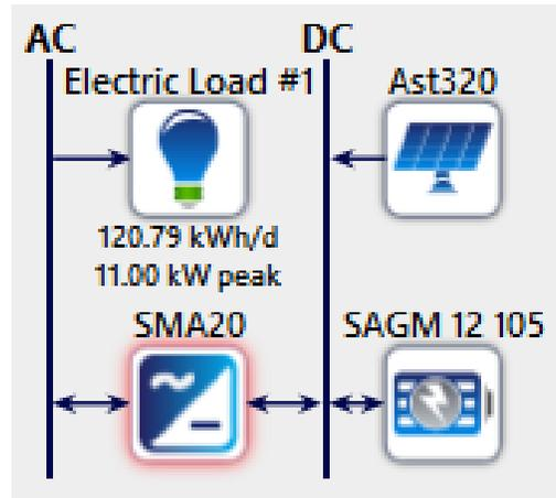
Figure 18: Proposed PV based water pumping system
