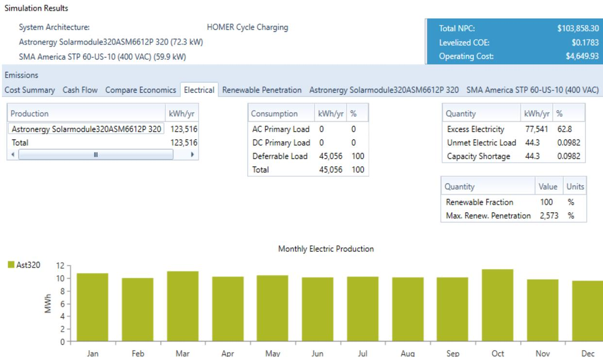
Figure 51: Simulation details for the proposed system with a water tank
