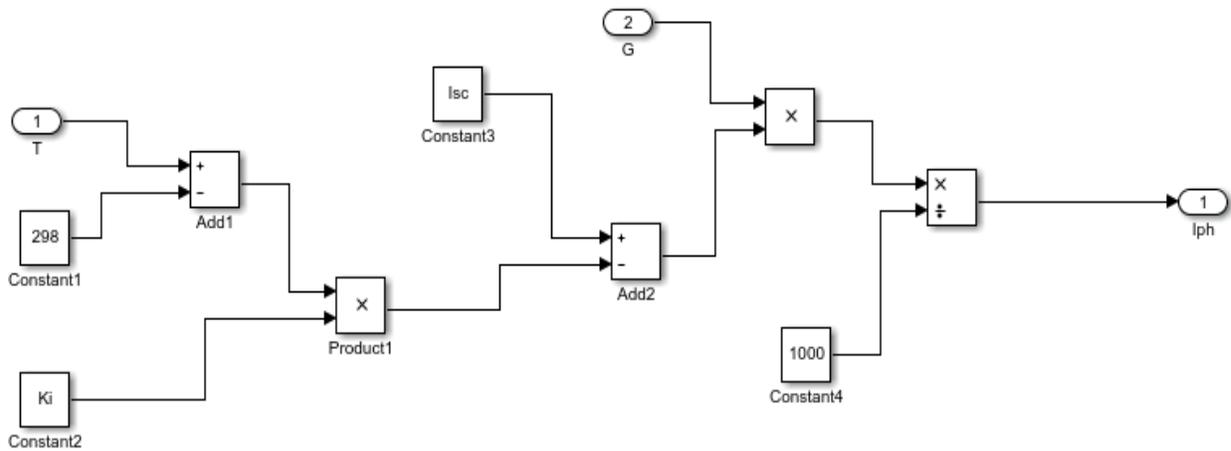
Figure 28: Photo-Current Equation modeled in MATLAB/Simulink
