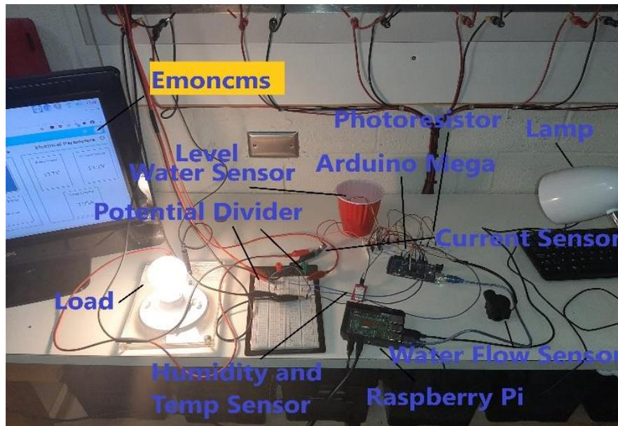
Figure 58: Prototype of Proposed SCADA system in Lab
