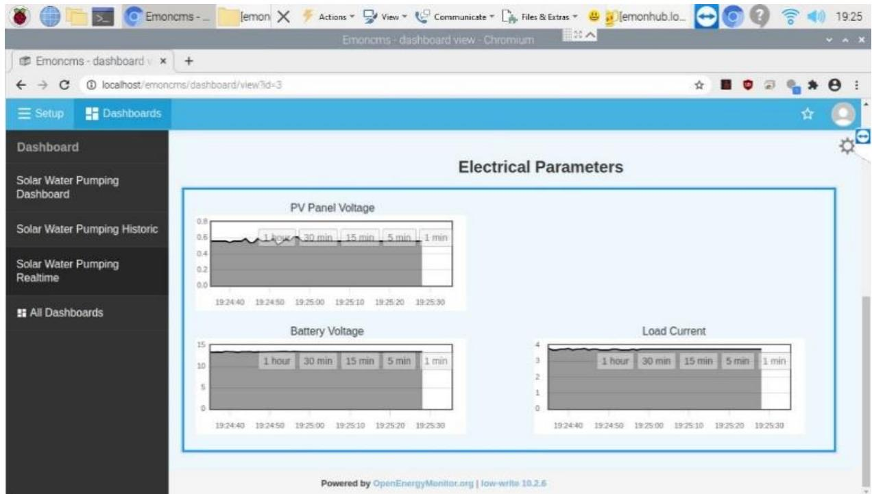
Figure 64: Real time Emoncms Dashboard for a solar water pumping system (Electrical Parameters)
