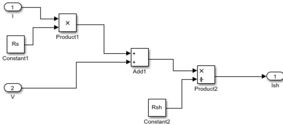
Figure 29: Shunt Current Equation modeled in MATLAB/Simulink
