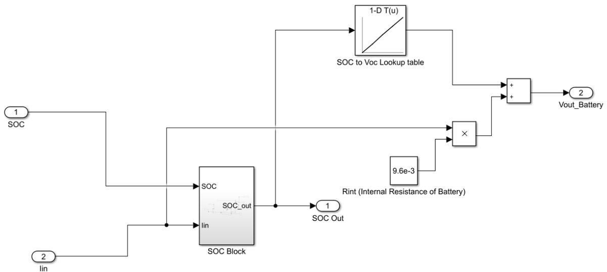
Figure 35: Battery Model in MATLAB/Simulink
