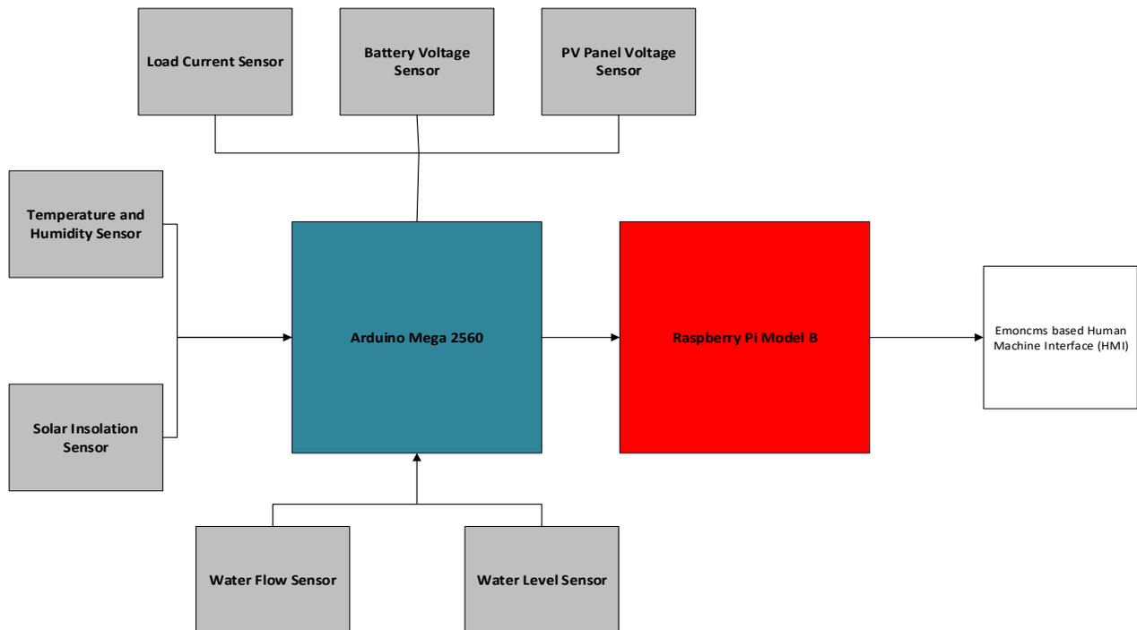
Figure 55: Proposed SCADA system for Solar Water Pumping System
