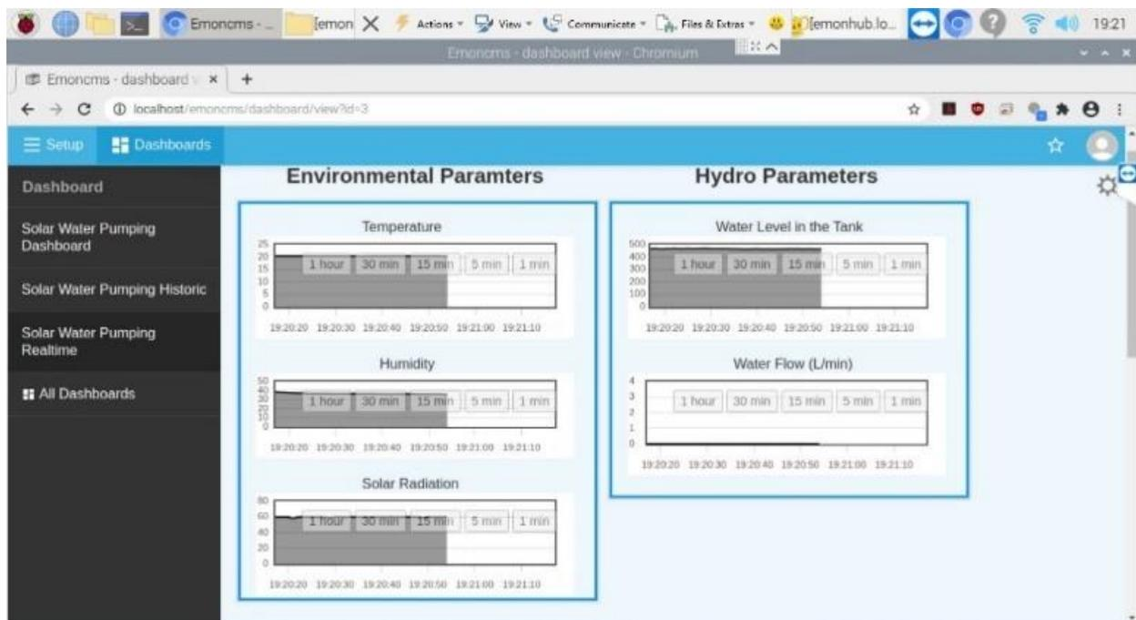
Figure 63: Real time Emoncms Dashboard for a solar water pumping system (Environmental and hydro Parameters)
