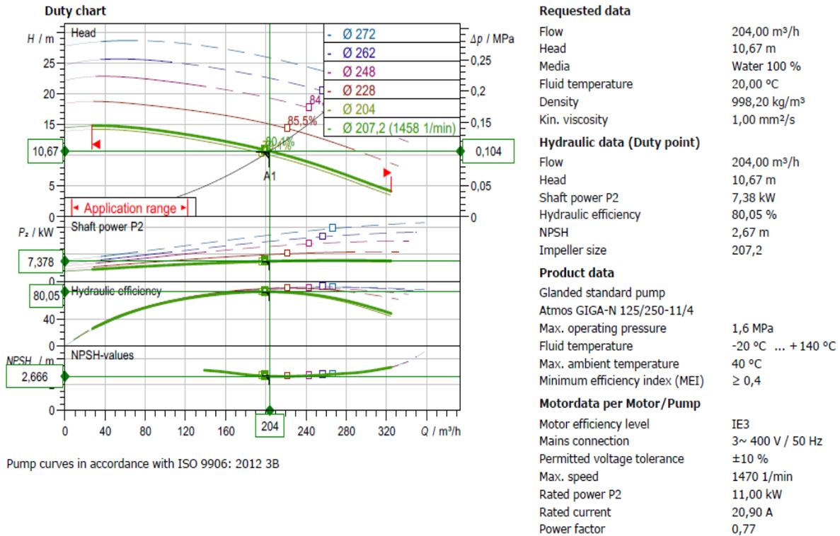
Figure 17: Selection parameters that led to motor selection
