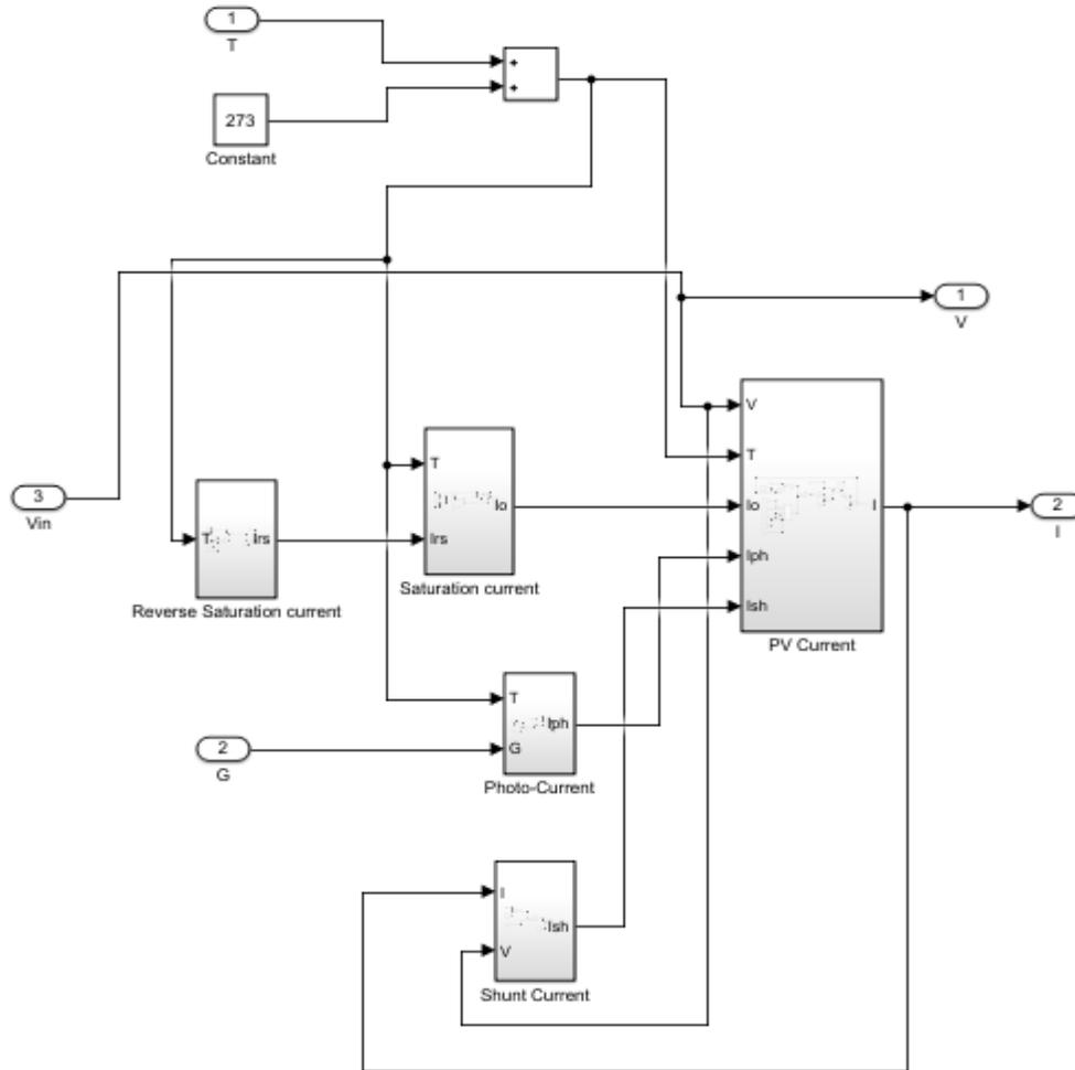
Figure 31: the Overall PV cell model in MATLAB/Simulink
