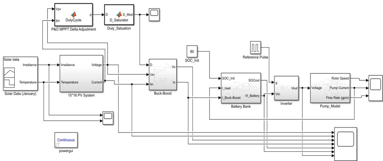
Figure 23: Dynamic Model of proposed PV based water pumping system with battery bank
