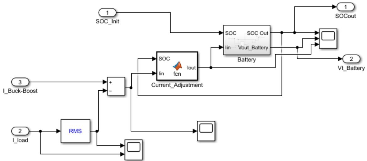
Figure 37: Inputs fed to battery bank Model
