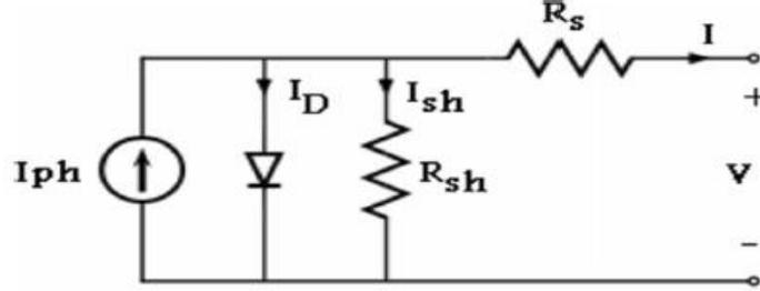
Figure 25: Single diode PV Cell Model
