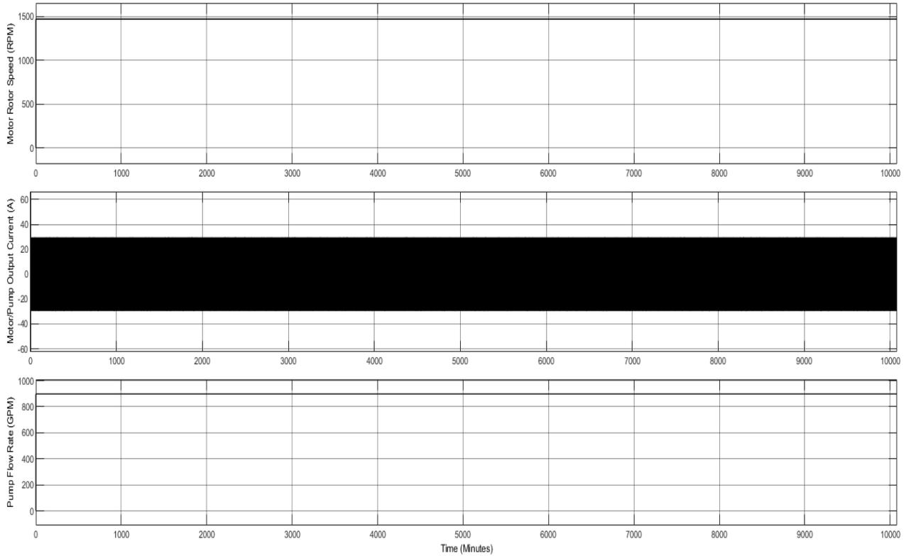
Figure 44: Simulation Results for Dynamic Modeling of Motor/Pump
