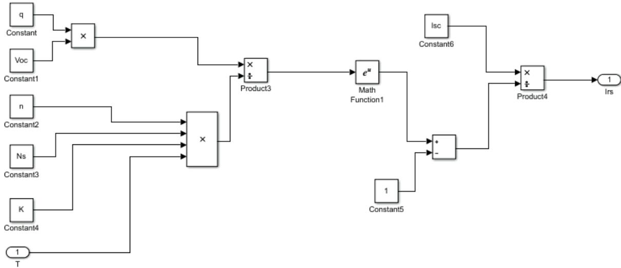
Figure 26: Reverse Saturation equation modeled in MATLAB/Simulink
