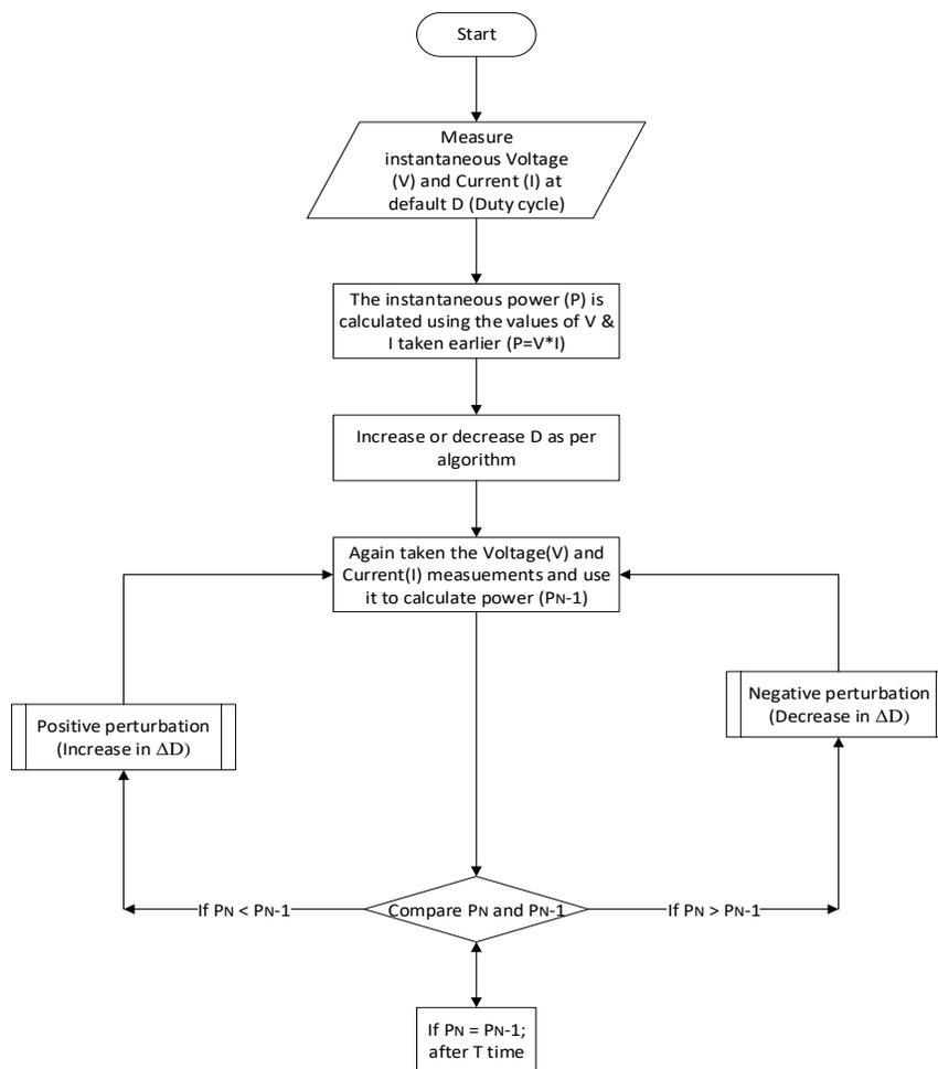
Figure 7: Flowchart of the algorithm for P&O MPPT Method
