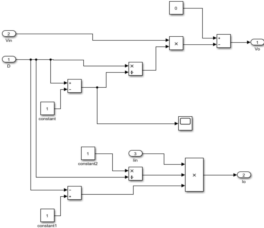
Figure 32: Buck-Boost voltage and current equations modeled in MATLAB/Simulink
