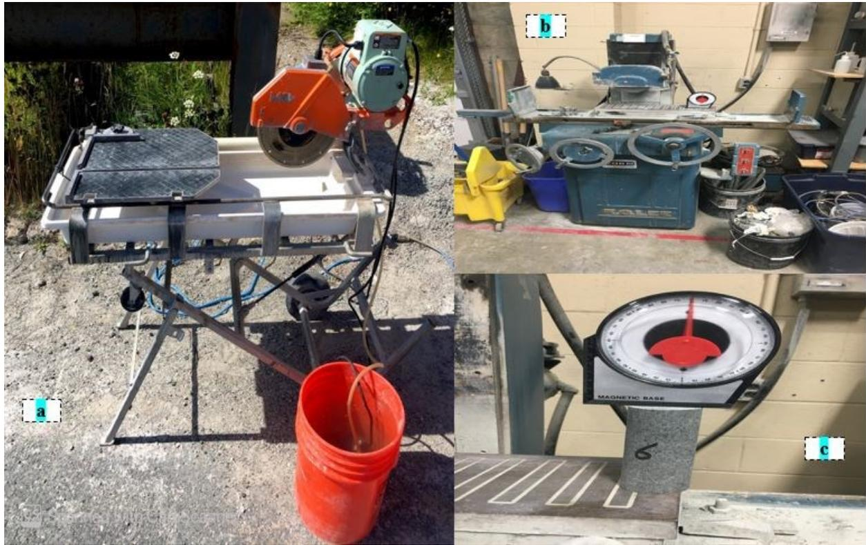
Figure 5.2: a. Core cutting saw; b. Grinder; c. Ensuring parallel edges of the core sample by grinder
