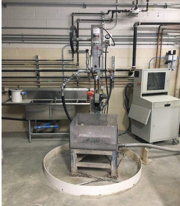
Figure 2.13: Small Drilling Simulator of DTL
