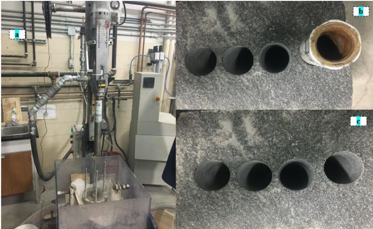
Figure 5.1: Coring for Granite Strength Test: a. SDS with coring bit; b. Granite Coring with bit ;
