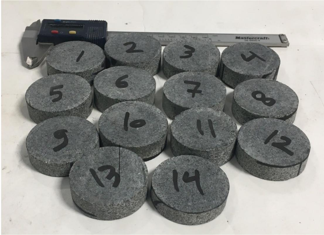
Figure 5.4: Granite samples for ITS tests according to D3967 - 16
