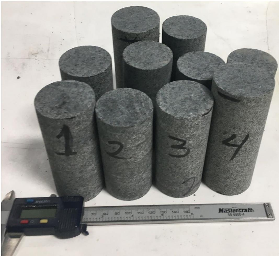
Figure 5.3: Granite samples for UCS test according to D7012-2014e1
