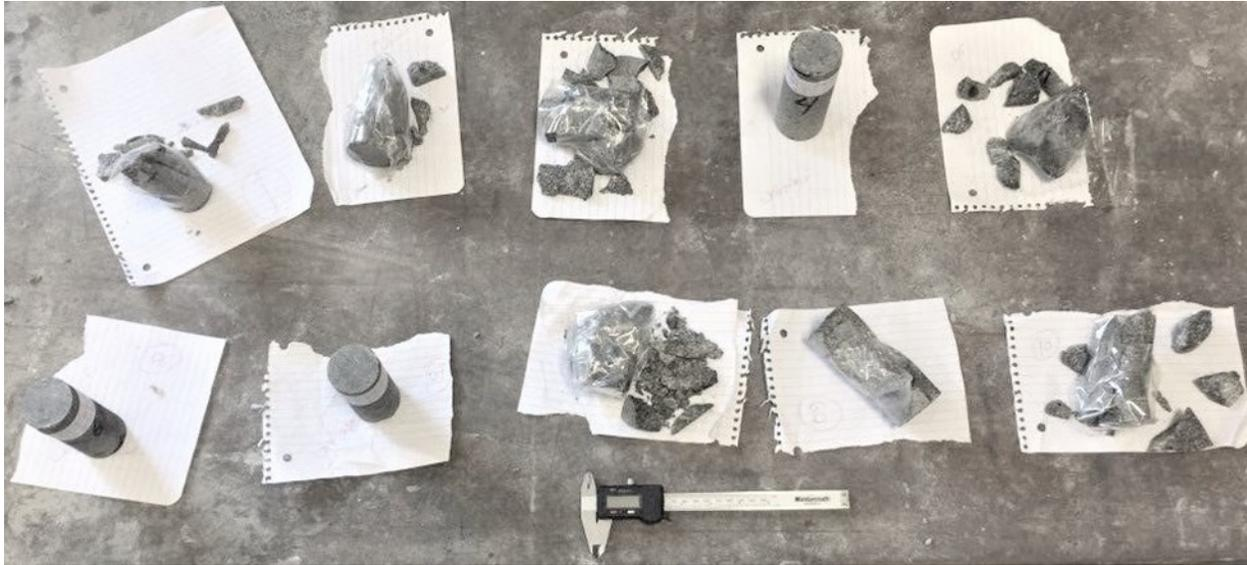
Figure 5.6: Granite samples after conducting the UCS test
