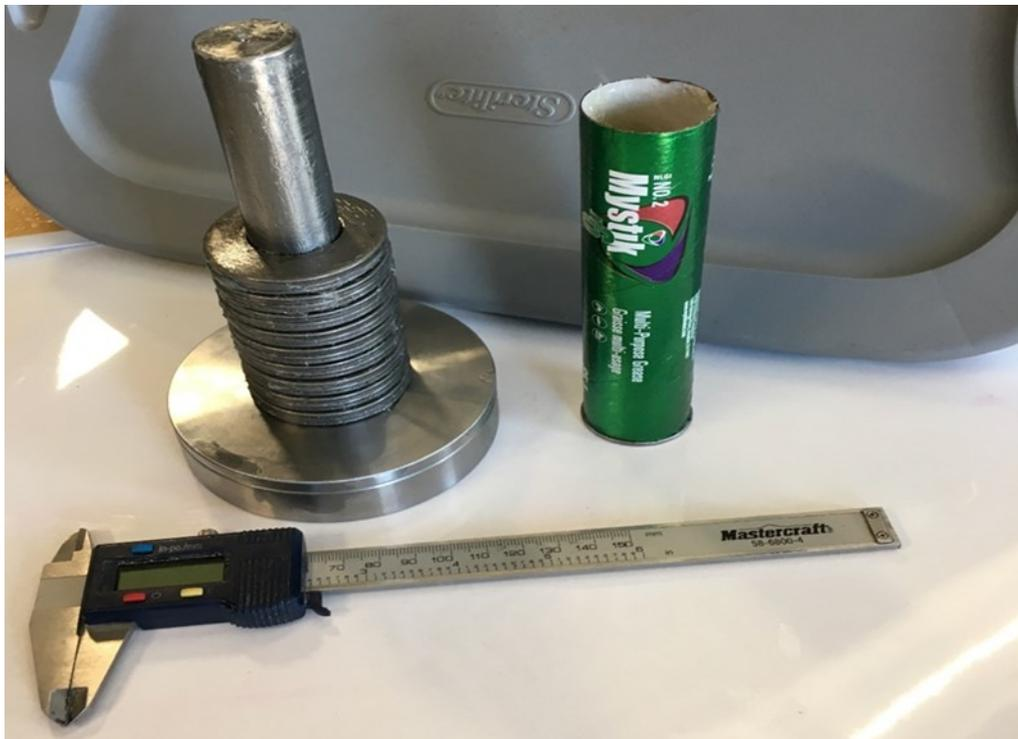
Figure 7.1: Commercial grease using 1-18 parallel springs configuration.
