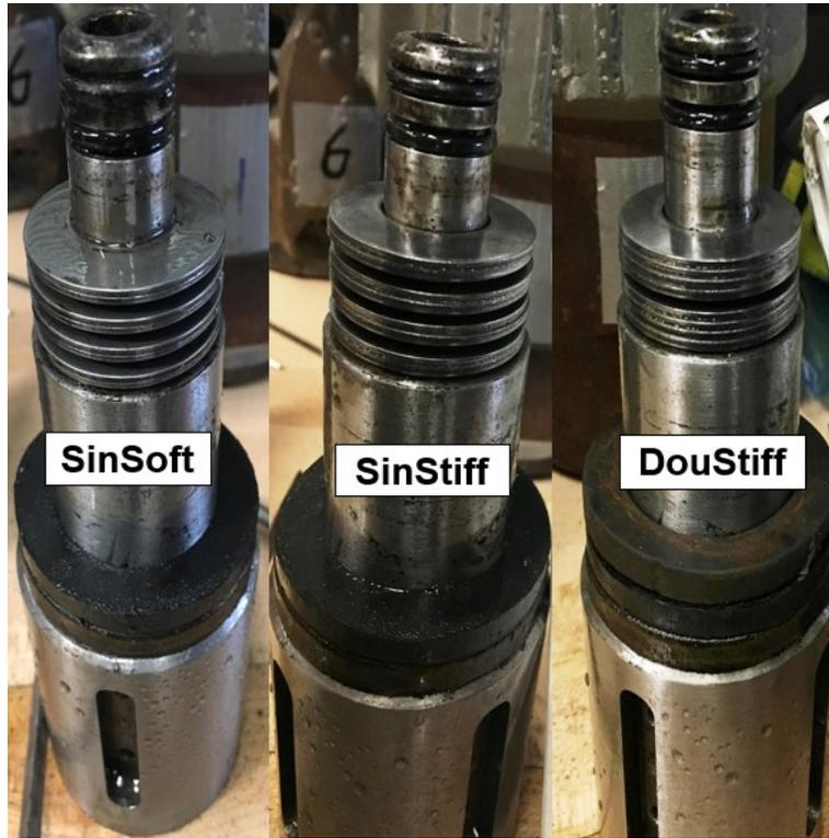
Figure 8.2: Configurations of the Belleville spring setting in the p-VARD tool, with 8 sets of single parallel soft springs (left), 8 sets of single parallel stiffer springs (middle) and 4 sets of double parallel stiffer springs (right).
