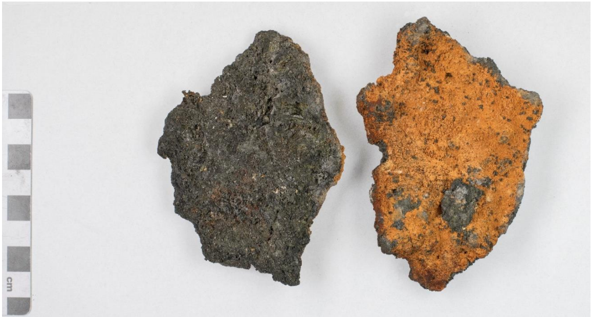
Hand samples for D1918-R13. Photograph showing fresh surface for one hand sample and the weathered surface for another. The respective surfaces are near identical for both pieces.
