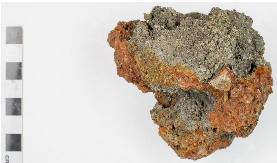
Hand sample for D1920-R10. Photograph shows a contrast of fresh and weathered surfaces.
