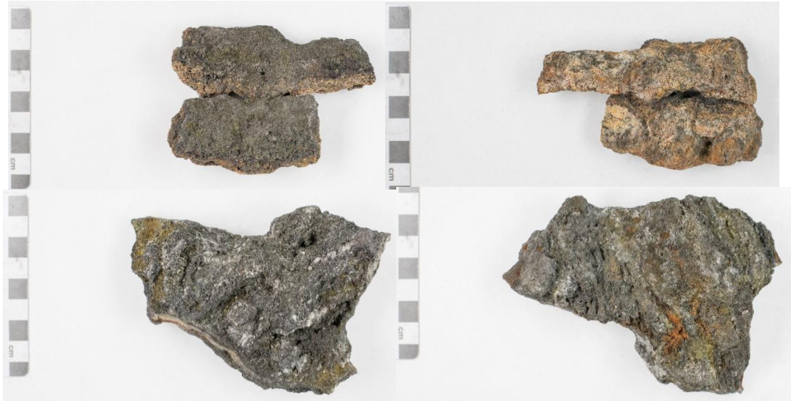
Hand samples for D1919-R6. Top left and right photographs show fresh and weathered surfaces for D1919-R6A, respectively. Bottom left and right photographs show two sides of D1919-R6B, largely consisting of fresh sulphide chimney material.
