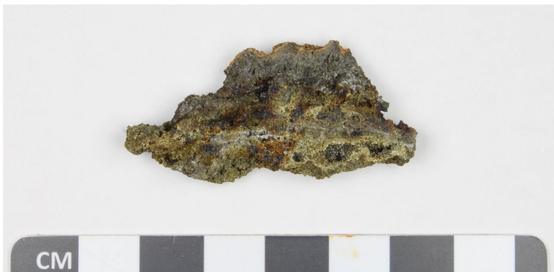
Thin section slab for D1918-R11. Thin section was cut from this face. “Peacock” iridescence is clearly visible in the chalcopyrite-rich zone.
