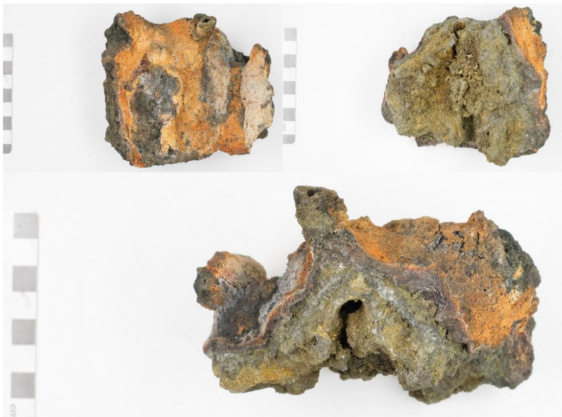
Hand sample for D1918-R8. Top left and right photographs show the vent exterior and interior, respectively. Bottom photograph shows a top-down view, highlighting the mineral zoning from interior to exterior.
