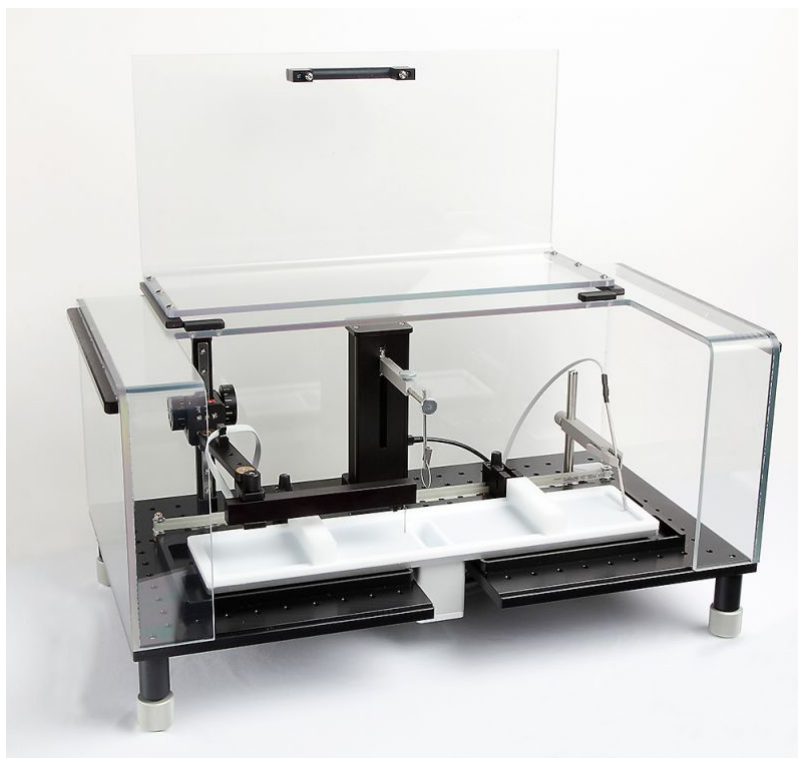
Figure 4.1: A typical depiction of the Langmuir-Williams surface balance. The Langmuir-Williams surface balance is characterized by a trough (white area) onto which the film spread, two moving barriers (the two white rods at each end), the pressure sensor at the center of the trough and a temperature sensor located at the far right. The box covering ensures resistance to shake and fluctuation to temperature.
