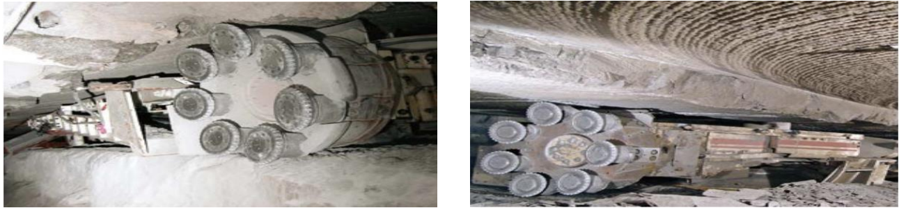
Fig 9. With the use of reef miner cutting machines the piston can be separated from the surrounding rock [7].
