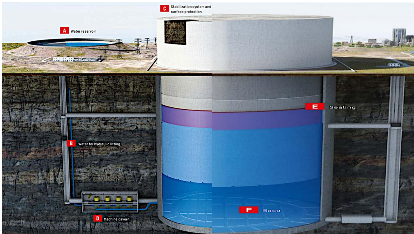
Fig 14. A Complete set up of Hydraulic Rock Energy Storage System [7].
