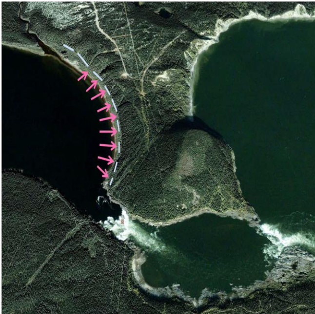
Fig. 2. Aerial view of Muskrat Falls on September 27, 2004. The North Spur Ridge, susceptible to a possible dam breach, is located in the centre of the picture just above the falls and the Rock Knoll granite cliff [9].
