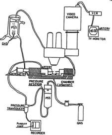
of gravity due to an elevated main reservoir and a faucet mounted aspirator. Helical coils of plastic tubing carried the Krebs saline through a warming jacket containing circulating water at 37°C. The water was warmed with a heater (Haake, model DI;Berlin) and circulated with a peristaltic pump (Watson -Marlow Limited, H.R. Flow Inducer, England).
