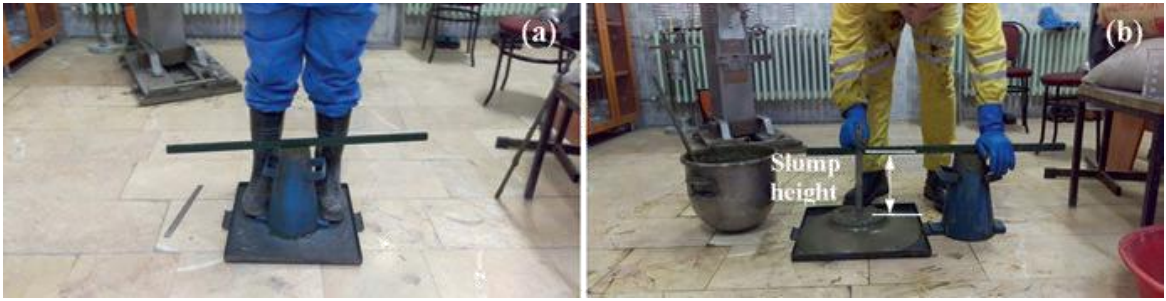
Figure 3 Schematic of the cone slump test (Erol Yilmaz and Mamadou Fall, 2017)
