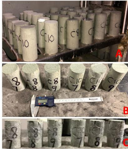
Figure 28-A) Samples while in the moisture room, B) and C) one set of samples before testing and after, respectively
