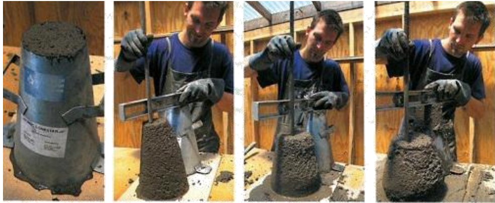
Figure 11-Slump procedure
