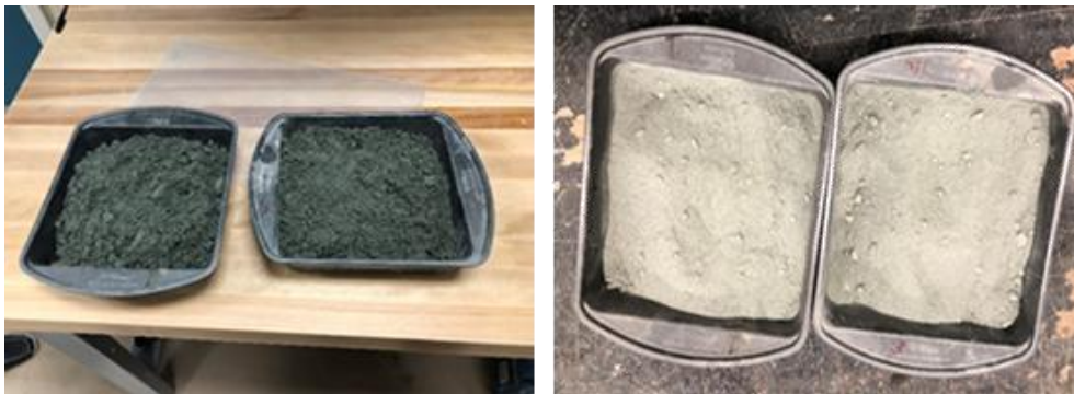
Figure 13-Tailings before (left) and after (right) drying
