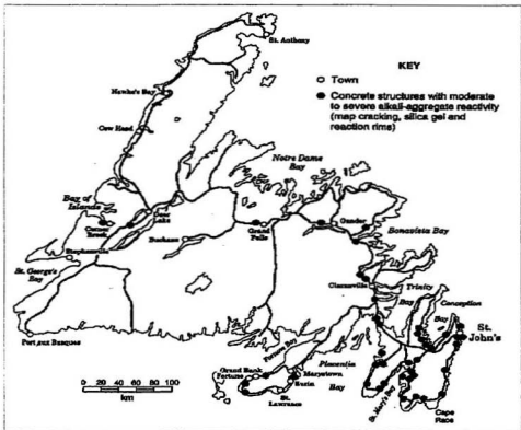
Figure 1 - Concrete structures with moderate to severe deterioration caused by AAR (Bragg, 1996)
