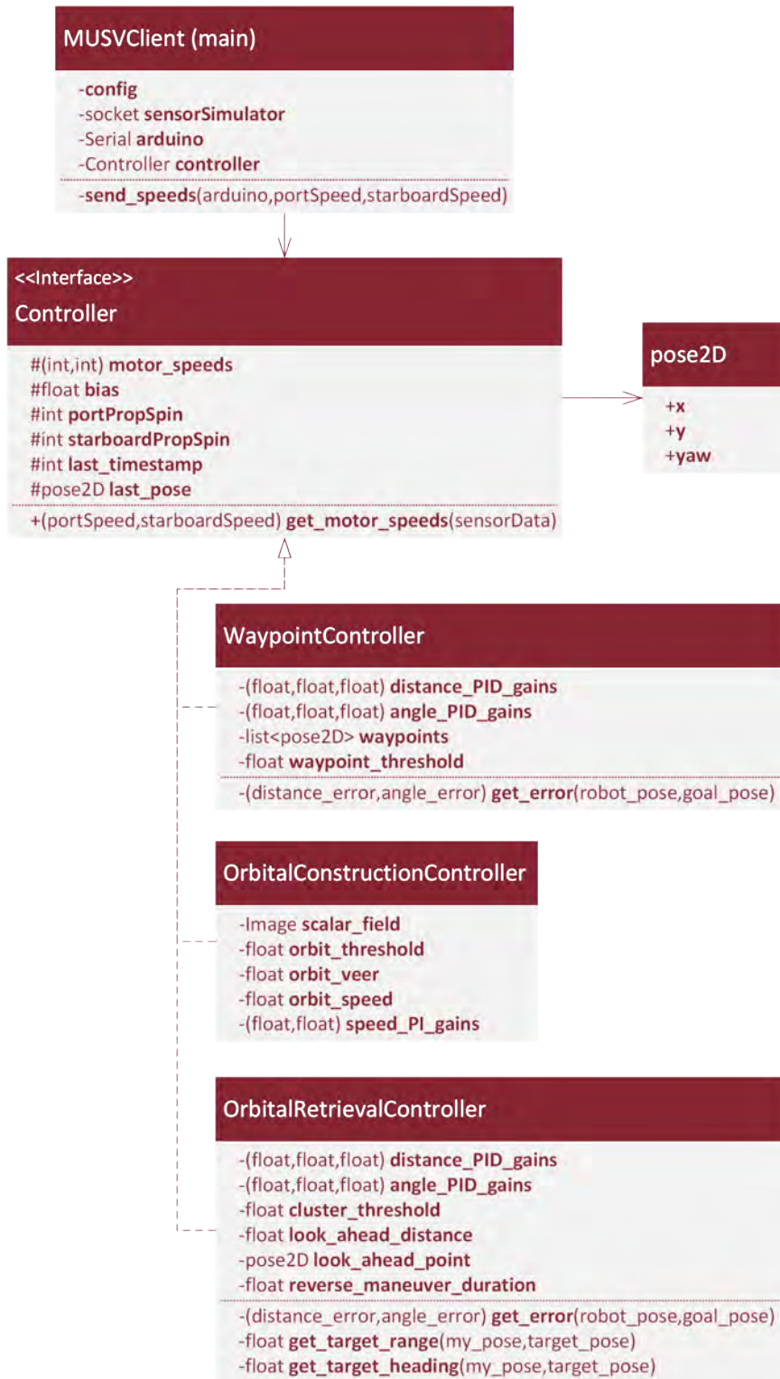
Figure 4.9: MUSVController Simplified Class Diagram
