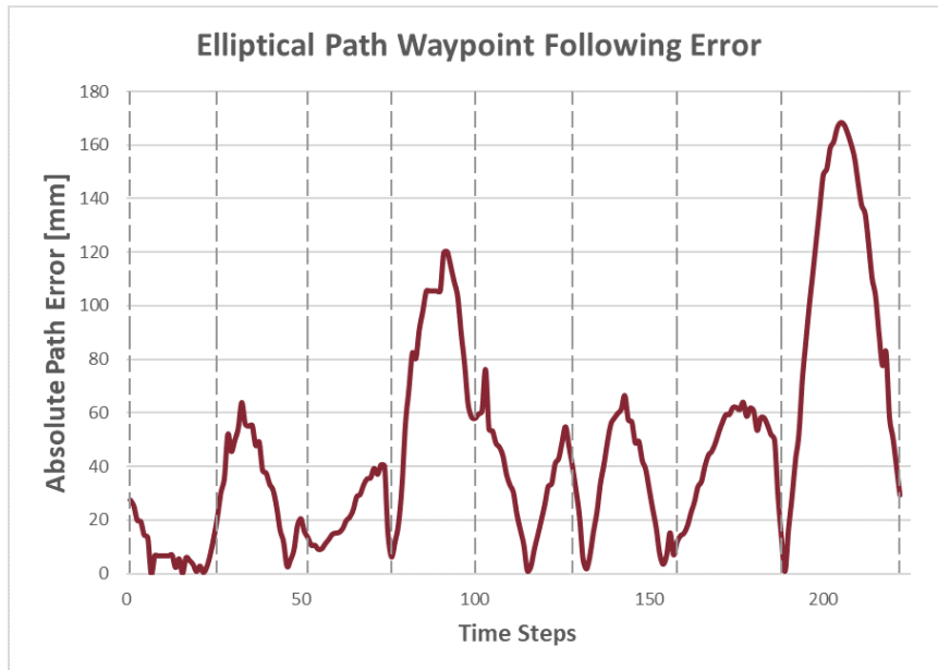
Figure 5.4: Elliptical Path Test Trajectory Error Plot
