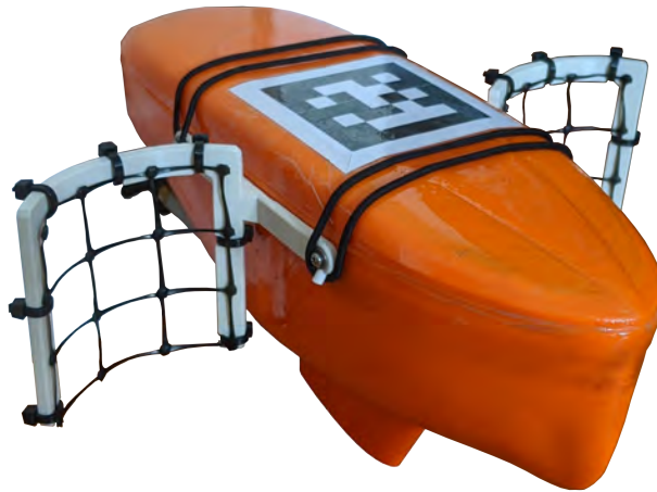
Figure 3.8: microUSV equipped with nets for contaminant clustering experiments
