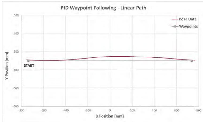
Figure 5.2: Linear Path Test Trajectory Plot
