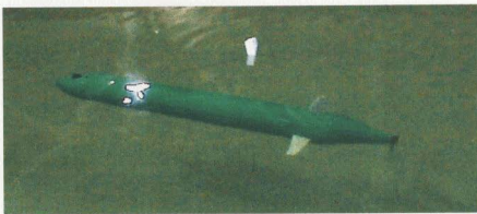
Figure 7.1.2: C-SCOUT operating entirely submerged.
