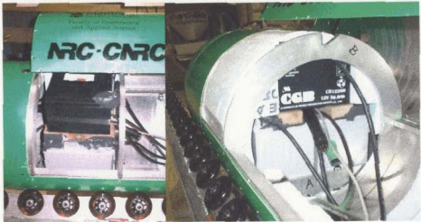
Figure 6.2.2: Battery stacking arrangement. Note cable tunnel between two lower batteries.
