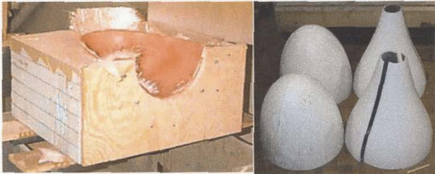
Figure 3.6.1: GRP being laid up in the nose mold (left) and multiple noses and tails (right)
