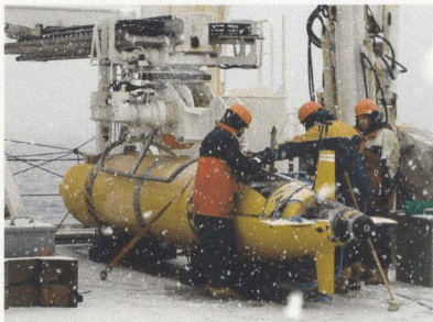
Figure 1.2.2: The AUV AutoSub. Again note the large vehicle and complex handling system required. Courtesy of Southampton Oceanography Centre, UK.
