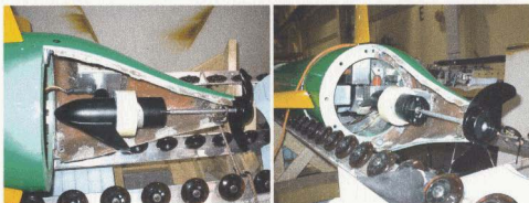
Figure 4.1.4: Minnkota 35T Trolling Motor mounted in the tail of C-SCOUT with the two-bladed Weedless Wedge propeller attached.
