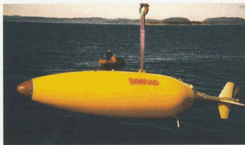
Figure 2.3.2: The Norwegian AUV, Hugin (Courtesy of Kongsberg-Simrad)
