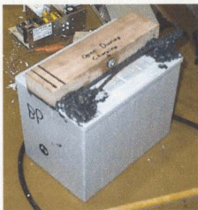
Figure 3.7.5: Renshape box over battery vents. Note screw to allow venting during charging.
