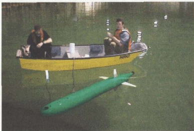
Figure 7.1.1: C-SCOUT being controlled through an Ethernet umbilical from a laptop and joystick inside the rowboat.
