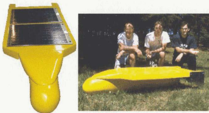
Figure 3.7.2: The Solar AUV, developed by the Autonomous Undersea Systems Institute of the United States. At the right, the solar panels have not yet been installed. (Courtesy of MSEL, 2000)
