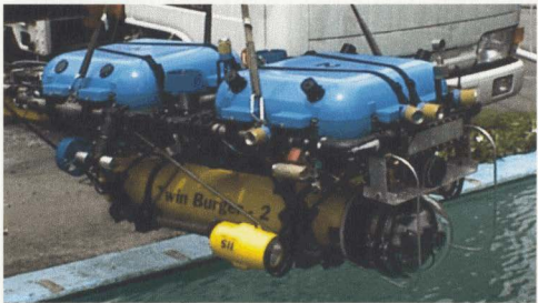
Figure 2.3.1: The AUV Twin Burger 2 by URA Laboratory, Institute of Industrial Science, University of Tokyo, Japan. Note the hydrodynamically inefficient form common to short-range AUVs.
