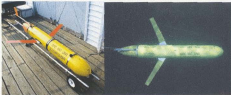
Figure 3.7.3: The ocean thermal energy powered SLOCUM has a range of 40,000 km over a period of 5 years. (Courtesy of Webb Research Corporation, 2001)
