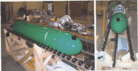
Figure 6.1.1: C-SCOUT Carriage. Note the three rails of inline-skate wheels used to align and hold the modules during modification and re-assembly.
