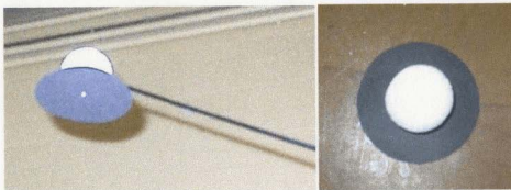
Figure D.3.1: Styrofoam tracking spheres mounted on carbon-fibre rods with black construction paper saucers for consistent image tracking.
