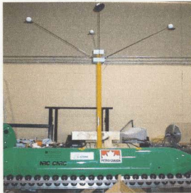
Figure D.2.1: The streamlined mast attached to the AUV C-SCOUT with tracking spheres and wireless Ethernet adapter mounted.
