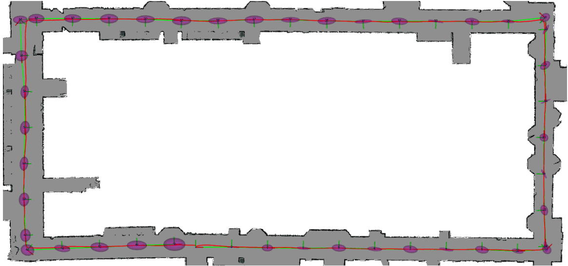
Figure 5.16: Error ellipsoids for a confidence of 99% (3 standard deviations)
