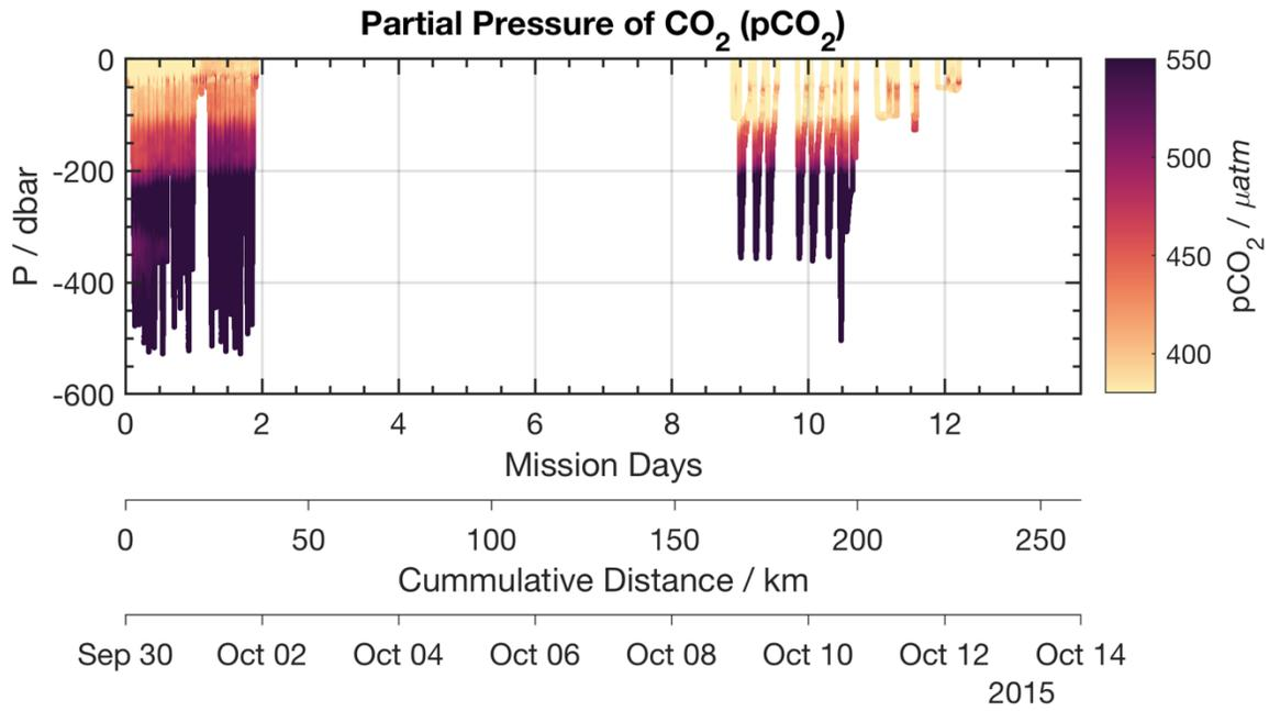
**Figure 4.14.3. Collected prototype Aanderaa CO<sub>2</sub> Optode data from the deployment. Some basic corrections have been done to correct the data for conditioning and sensor lag, but the data are not validated. A basic surface correction has been applied to bring the data closer to the mean atmospheric CO<sub>2</sub> values in October 2015. This is the best performance of this sensor in the 3 glider deployments.**
