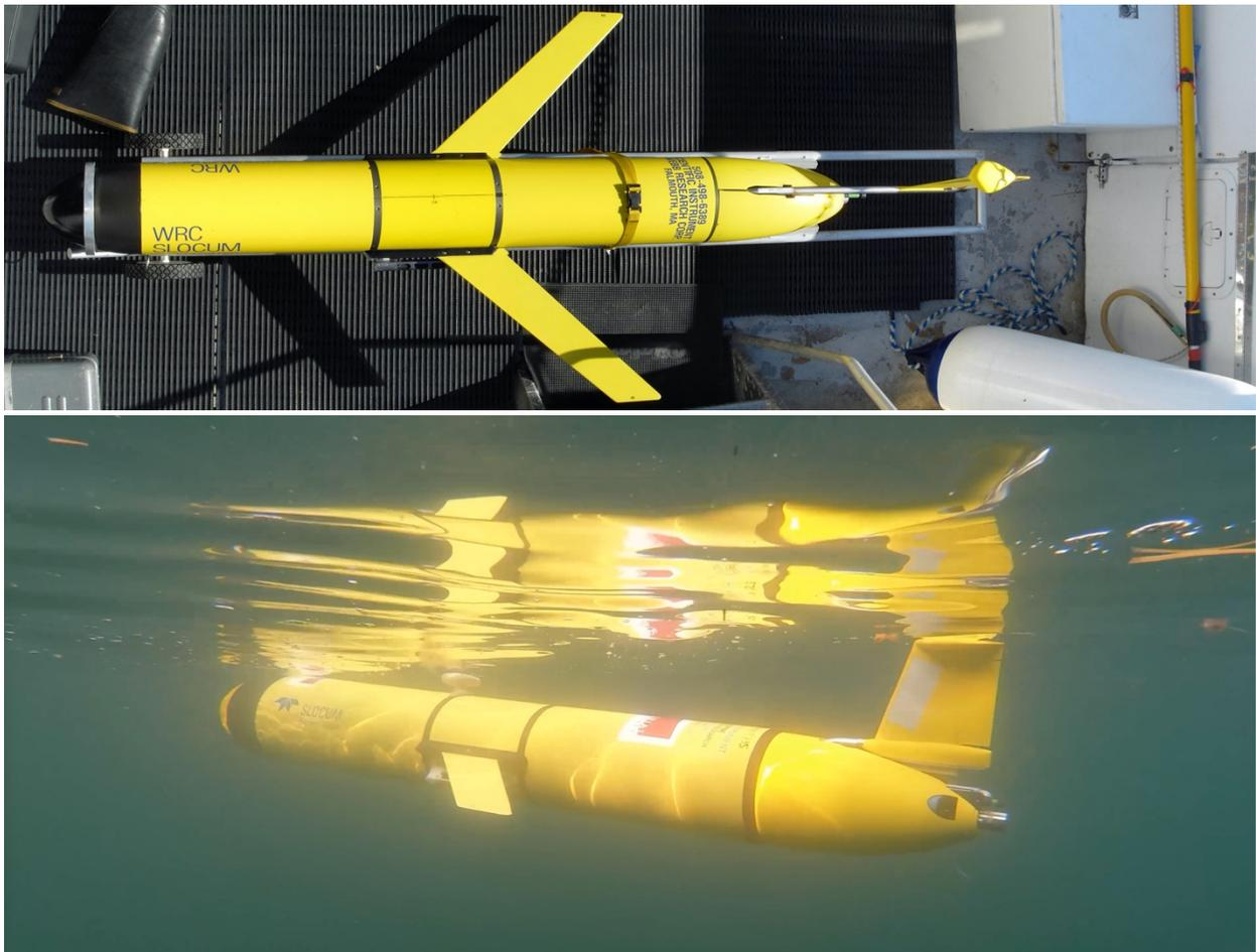
**Figure 1.1 Example of early MUN Slocum Glider (Unit 049) with unpumped CTD (SBE41) and a later version G2 1000m Slocum Glider (Unit 473) showing an Oxygen Optode (ADI 4831) and pumped CTD (GPCTD).**
