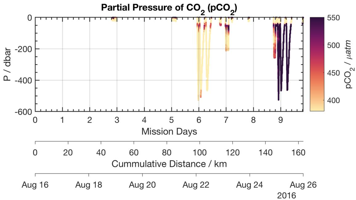
Figure 4.15.3. Collected prototype Aanderaa CO<sub>2</sub> Optode data from the deployment. Some basic corrections have been done to correct the data for conditioning and sensor lag, but the data are not validated. A basic surface correction has been applied to bring the data closer to the mean atmospheric CO<sub>2</sub> values in October 2016.
