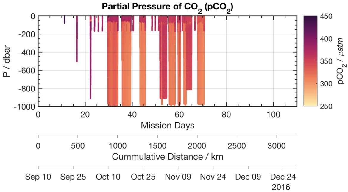
**Figure 4.16.3. Collected prototype Aanderaa CO<sub>2</sub> Optode data from the deployment. Some basic corrections have been done to correct the data for conditioning and sensor lag, but the data are not validated. A basic surface correction has been applied to bring the data closer to the mean atmospheric CO<sub>2</sub> values in October 2016. Constant oxygen and CO<sub>2</sub> values with depth are artefacts from the glider thruster.**
