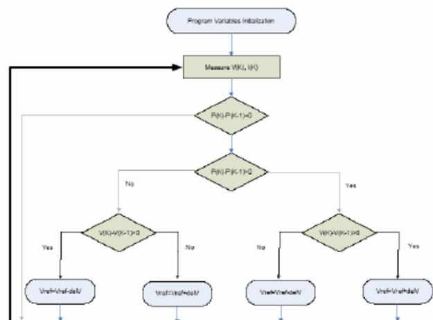
Figure 15: Flowchart of the MPPT control As the traditional dc/dc converter has negative impedance characteristic, the solar array is required to operate on the right side of the curve to perform the tracking process. The control flowchart in figure 15 illustrates the details of decision processes. If the given perturbation leads to an increase in array power, the next perturbation is made in the same direction. In this way the maximum power tracker seeks the maximum power point continuously.
