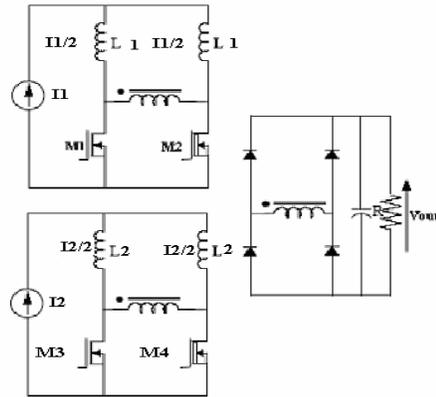
Figure 8: Multi-input current source half-bridge converter
