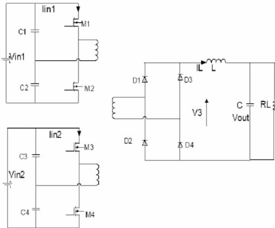
Figure 4: Multi-input half bridge converter
