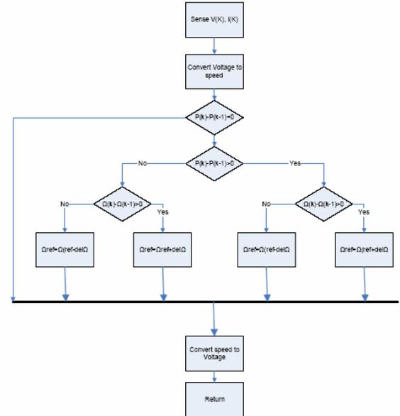
Figure 17: Basic flow chart of the MPPT control for Wind energy conversion system
