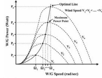
Figure 16: Power curves at various wind speeds
