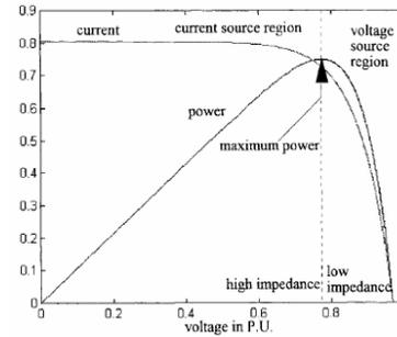
Figure 14: Solar array characteristic curve [11] proposed in a software program with a self tuning function. The program automatically adjusts the array reference voltage and voltage step size. The problem- incapable of tracking maximum power in fast changing environment, with the method is wished to overcome by increasing sampling frequency.
