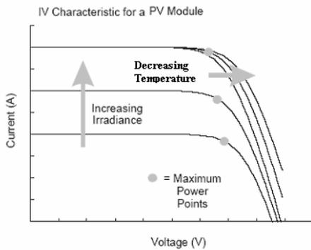
Figure 13: Typical IV characteristic of a crystalline solar PV module
