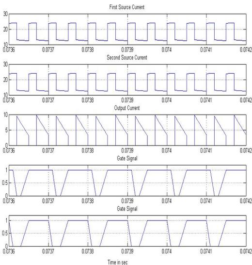
Figure 10: Simulation results of MI CS converter (case4) operating at 70% duty cycle whereas the switches in the second-input stage are operating at 60% duty cycle. When the
