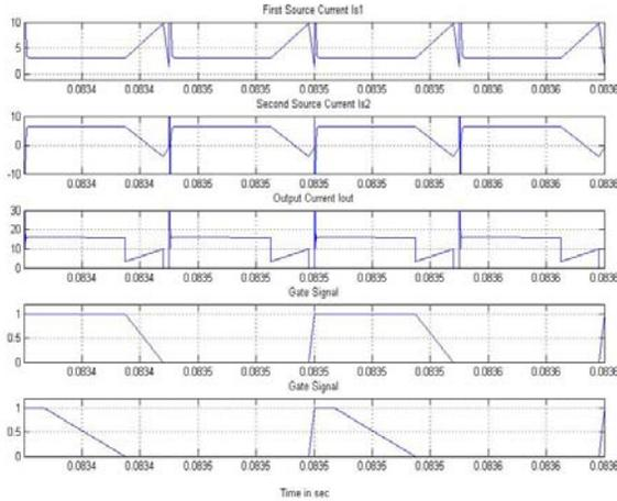
Figure 6: Simulation result –currents for case2 direction of the source current and feedback current are same, so current is adding up in input stage 1.
