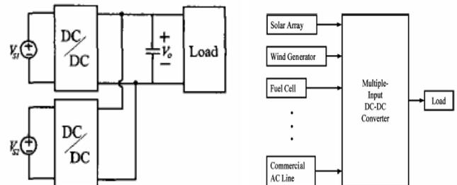
Figure 2: Basic configuration of parallel operation of converters and MI converter
