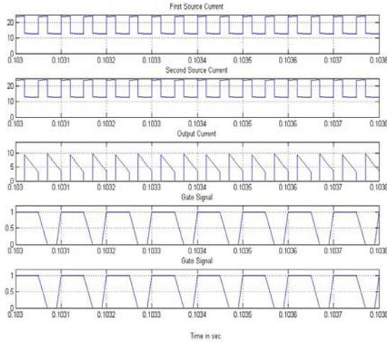
Figure 9: Simulation results of CS converter (case 3) in a boost phase or free wheeling stage. When only one switch is closed, the converter is said to be in a powering phase as current is delivered to the output rectifier. The same operation occurs in the input stage 2. Figure 9 shows the simulation results.
