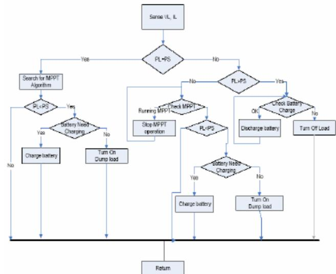
Figure 12: Supervisory controller flow chart
