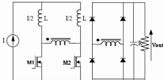
Figure 7: Dual of the half bridge converter
