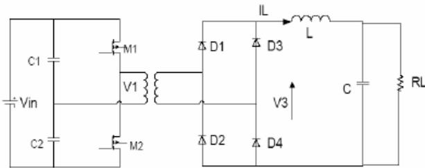
Figure 3: Half bridge push-pull converter
