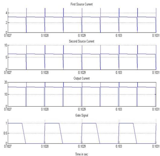
Figure 5: Simulation results of MI half bridge converter (case1) Figure 5 is the current wave shape for different stage with gate signal for M1. Here 48% duty cycle is considered.
