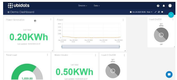
Figure 7 Ubidots Dashboard prototype for the proposed SCADA system.
