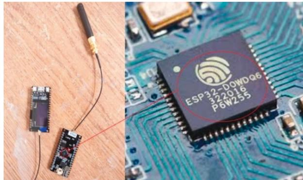
FIGURE 13: ESP32 with LoRa module used for AES implementation.
