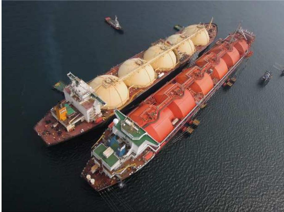
Figure 1.1: Side-by-Side Offloading Operation ([www.royalhaskoningdhv.com](http://www.royalhaskoningdhv.com))
