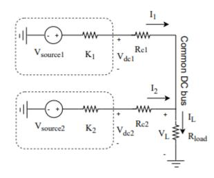
Figure 2. Thevenin equivalent model for two parallel-connected converters.
