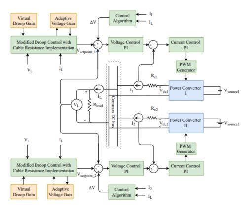
Figure 9. Block diagram of the alternative droop control method.
