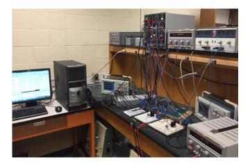
Figure 17. Prototype parallel-connected DC-DC boost converters system.
