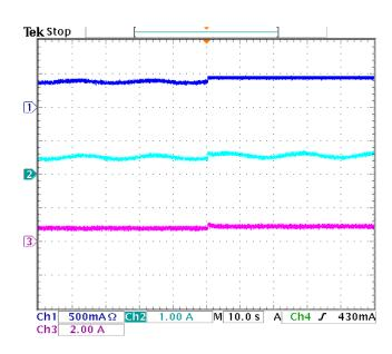
Figure 18. Experimental results of load current sharing accuracy for step change in the load current.
